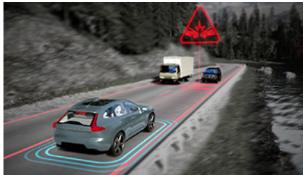
Oncoming Mitigation by Braking A Volvo Cars safety world first, this innovation can detect vehicles heading towards you on the wrong side of the road. If a collision can't be avoided, it can brake your car automatically and tighten the optional prepared front safety belts in order to help reduce the effect of a collision.
