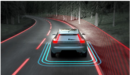
Run-off road Mitigation Stay safely on the road with this Volvo Cars safety innovation. If Run-off road Mitigation detects you're about to leave the road unintentionally, it can provide steering input and, if necessary, brake support to help guide you back on track.
