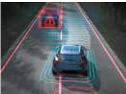
Oncoming Lane Mitigation Using automatic steering assistance, this system helps you avoid collisions with oncoming vehicles. If you drift across the lane markings in the way of an oncoming vehicle, your car steers back.
