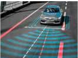
Lane Keeping Aid If you're about to cross a lane marking unintentionally, the Lane Keeping Aid will gently steer your car back into its lane. If this is not enough or you keep steering across the lane markings, you'll be alerted with vibrations in the steering wheel.
