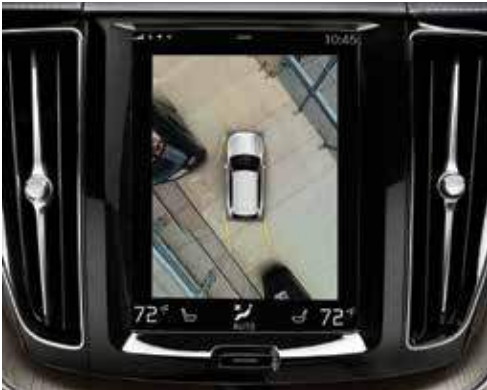
360° SurroundView Camera The 360° SurroundView Camera uses images from discreetly mounted cameras to create a bird's-eye view of your car and its closest surroundings. In the center display, you can see obstacles all around you, which makes it easier to park and maneuver in tight spaces.
