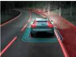
Run-off Road Mitigation Stay safely on the road with this Volvo Cars safety innovation. If Run-off Road Mitigation detects you're about to leave the road unintentionally, it uses steering input and, if necessary, brake support to guide you back on track.
