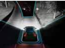
Full-LED Active High Beam Illumination To give you the best view, our Full-LED headlights allow you to drive with high beam on all the time, without dazzling others. It detects road users ahead of you and automatically shades the part of the high beam that would dazzle them.
