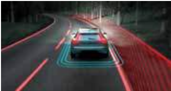
Run-off Road Mitigation Stay safely on the road with this Volvo Cars safety innovation. If Run-off road Mitigation detects you're about to leave the road unintentionally, it can provide steering input and, if necessary, brake support to help guide you back on track.
