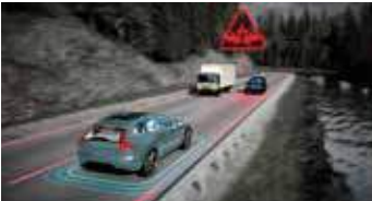
Oncoming Mitigation by Braking A Volvo Cars safety world first, this innovation can detect vehicles heading towards you on the wrong side of the road. If a collision can't be avoided, it can brake your car automatically in order to help reduce the effect of a collision.
