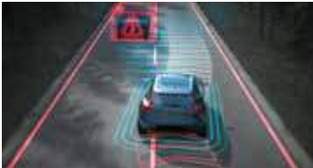
Oncoming Lane Mitigation If you drift across the lane markings and into the path of an oncoming vehicle, your car can alert you and gently help steer you back onto the correct path. This system does this using automatic steering assistance, helping you to avoid collisions with oncoming vehicles.
