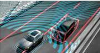
BLIS™ BLIS™ uses radar sensors at the rear of the car to monitor your surroundings, and can detect if vehicles have entered your blind spot or are approaching fast from behind. If you pull out into the path of an approaching vehicle it can also help alert you.
