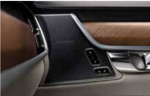
Harman Kardon® Premium Sound is developed together with the hi-fi specialists at Harman Kardon®. Powered by a 600W digital amplifier, the 14 speakers are tailored to the acoustics inside your Volvo and deliver a powerful, high fidelity surround sound experience. A unique sound processing software – Dirac® Unison Tuning – optimizes the response of each individual speaker as well as the speakers all together to ensure they perform in perfect harmony. So wherever you're seated, you and your passengers can enjoy a seamless first-class listening experience in all conditions and – not least – an extremely unified and tight bass sound.
