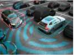
Cross Traffic Alert Cross Traffic Alert is included on all vehicles equipped with BLIS, and alerts you of crossing traffic from the sides when reversing out of a parking space.
