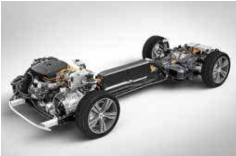
The S60 has been designed from the ground up with plug-in hybrid power in mind, so the batteries and electric motor are set lower in the chassis. This means more responsive, intuitive handling due to a lower center of gravity and more even weight distribution.
