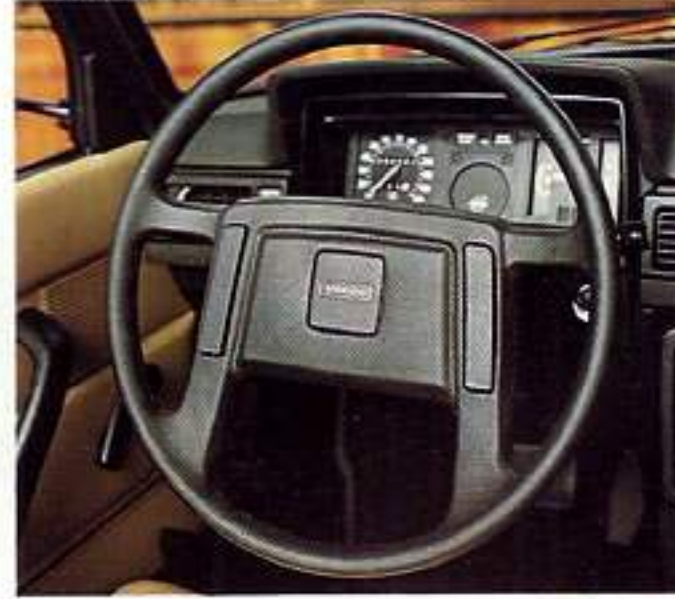
Padded safety steering wheel, variable-intensity illuminated instrumentation.
