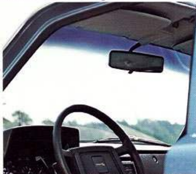
Tinted windshield with dark tint band, three-layer laminated "high-impact" design.
