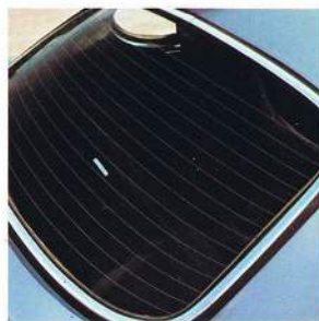
A grid of fine wires embedded in the rear window of the 1800E defrosts it electrically. The 1800ES uses the same system. It's standard equipment.
