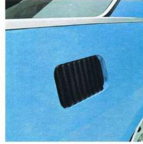
The flow-through ventilation system keeps air circulating in the car even when the windows are closed. The extractor vents are designed to let out air but not let any exhaust in.
