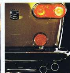
Four-way emergency warning flashers incorporated in turn indicators.
