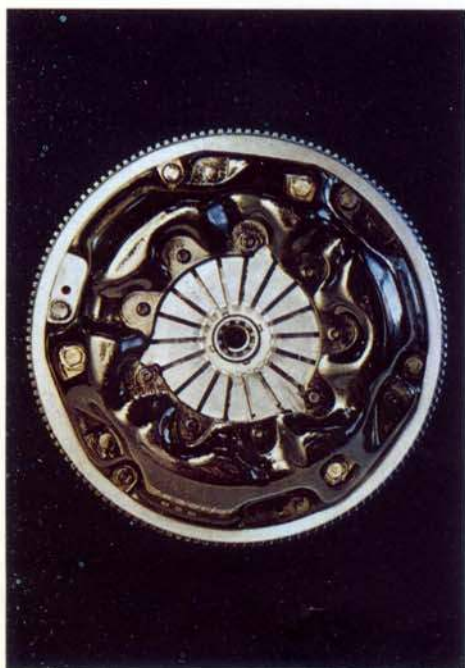
The diaphragm clutch requires less pedal pressure
