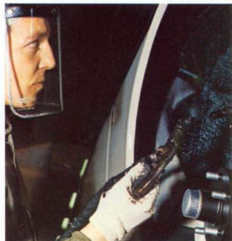
Comprehensive underbody sealing before the cars leave the factory
