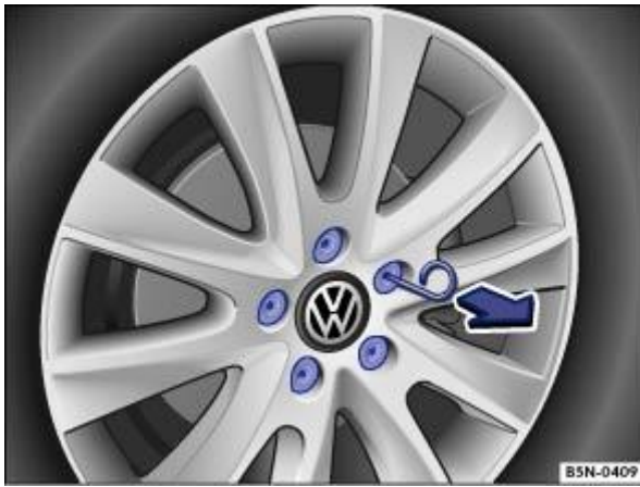
Fig. 202 Removing the wheel bolt caps.
