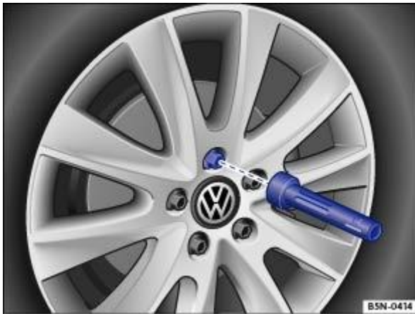
Fig. 207 Changing a wheel: removing the wheel bolts with the screwdriver handle.
