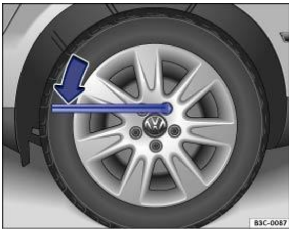
Fig. 203 Changing a wheel: loosening the wheel bolts.
