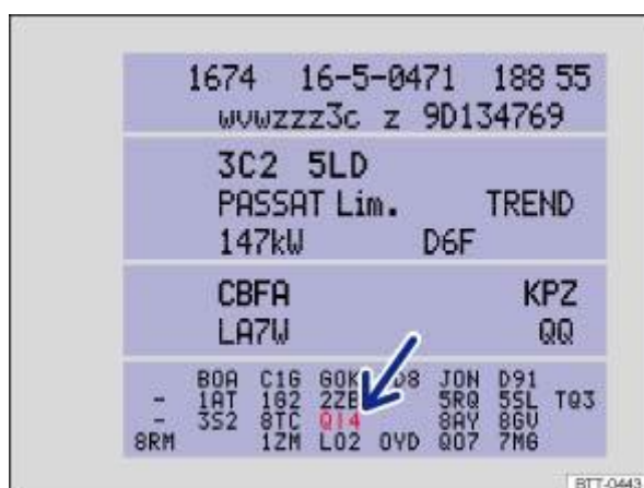
Fig. 210 Vehicle data sticker with PR number for the relevant service (illustration).
