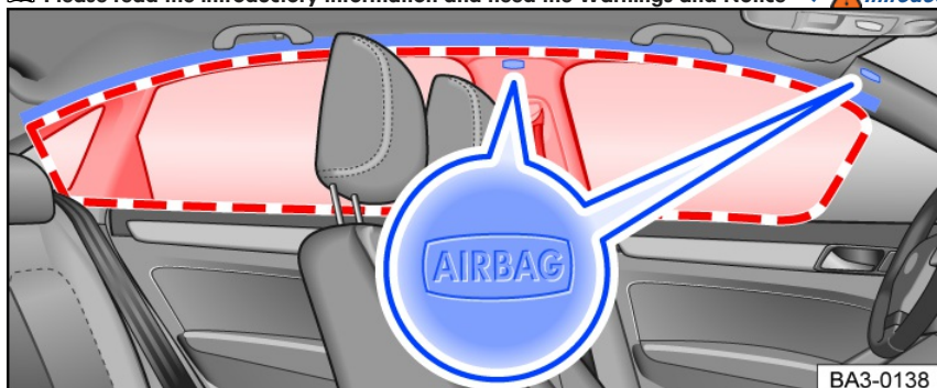
Fig. 31 On the left side of the vehicle: installation location and deployment zone of the Side Curtain Protection®.
