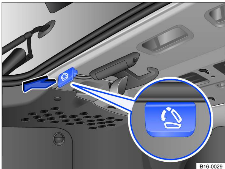
Fig. 65 In the luggage compartment: Remote release lever.
