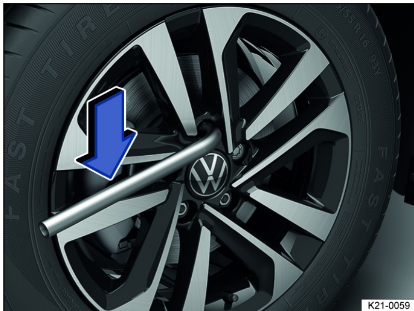
Fig. 161 Wheel change: removing wheel bolts with the lug wrench.
