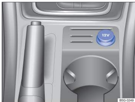
Fig. 138 In the lower center console: 12 Volt socket (vehicles with parking brake lever).
