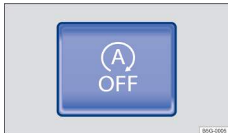
Fig. 99 In the lower center console: Button for the Start-stop system (if equipped).
