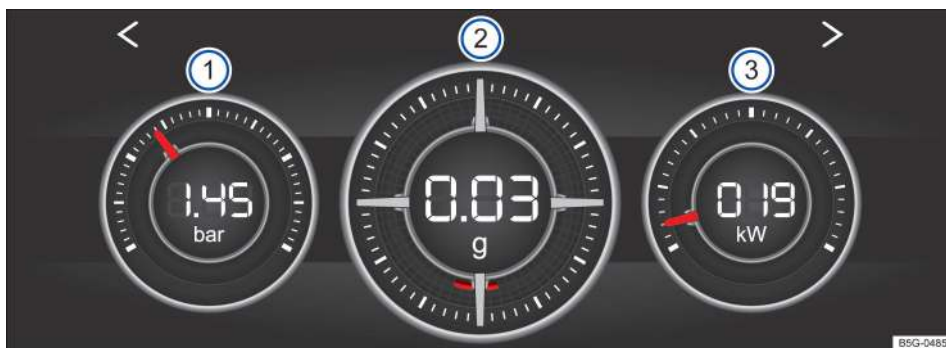
Fig. 18 In the Infotainment system: Performance Monitor sport gauges (if equipped). Gauges shown in the display may vary depending on configuration.
