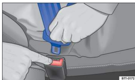
Fig. 29 Releasing the buckle tongue from the belt buckle.
