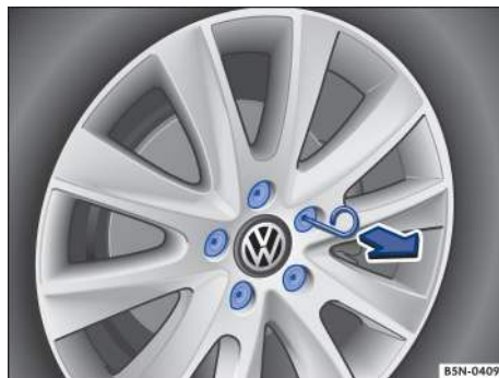
Fig. 184 Pulling cover caps off wheel bolts.
