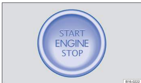
Fig. 97 In the lower center console: Starter button for the Keyless Access system.
