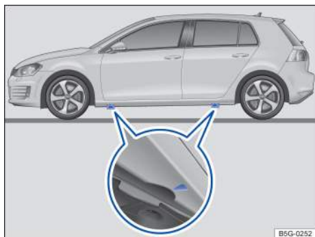
Fig. 189 Lift points for the jack.
