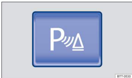
Fig. 116 In the lower center console: Button to switch the Park Distance Control system on or off.
