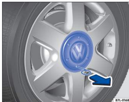
Fig. 181 Pulling the hubcap off.
