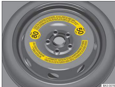
Fig. 179 In the luggage compartment: Compact spare wheel (label design may vary).
