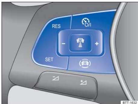
Fig. 110 Left-hand side of the multi-function steering wheel: Buttons for operating the Adaptive Cruise Control (ACC).
