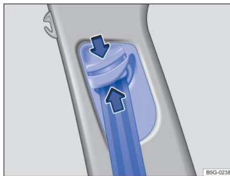
Fig. 32 Next to the front seats: Safety belt height adjuster.
