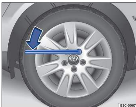
Fig. 185 Changing a wheel: Loosening the wheel bolts.
