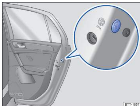
Fig. 55 On the front side of the rear passenger door: Manual lock, covered by a rubber seal.
