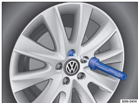
Fig. 191 Changing a wheel: Remove previously loosened wheel bolts using the screwdriver handle.
