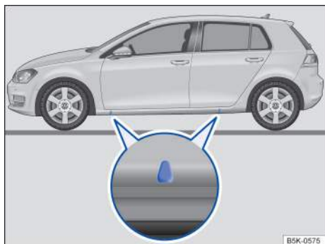
Fig. 187 Lift points for the jack.
