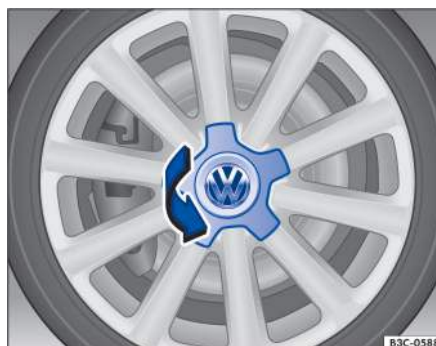
Fig. 182 Twisting the hubcap off.
