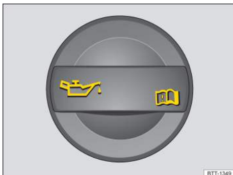
Fig. 171 In the engine compartment: Engine oil filler cap (cap design may vary depending on vehicle equipment).
