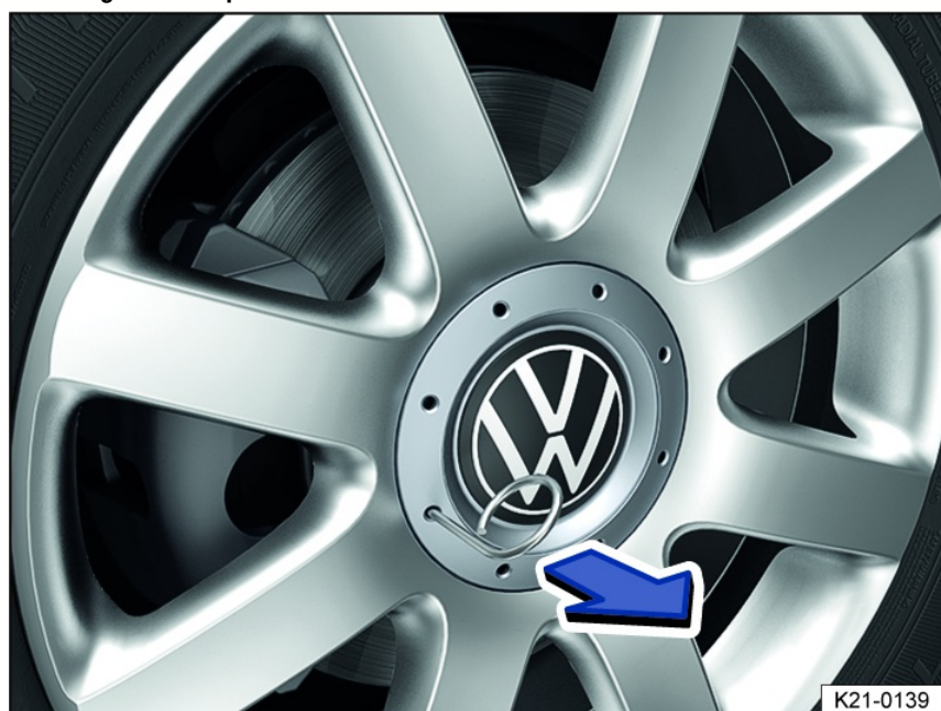
Fig. 152 Remove the hubcap.
