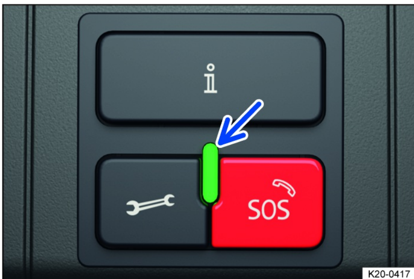
Fig. 39 In the roof console: controls for call services.
