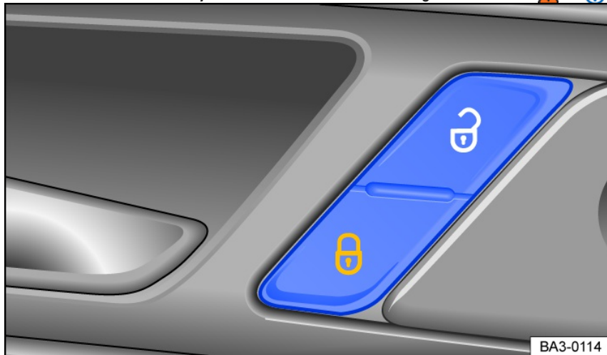
Fig. 45 In the driver's door: central locking button.
