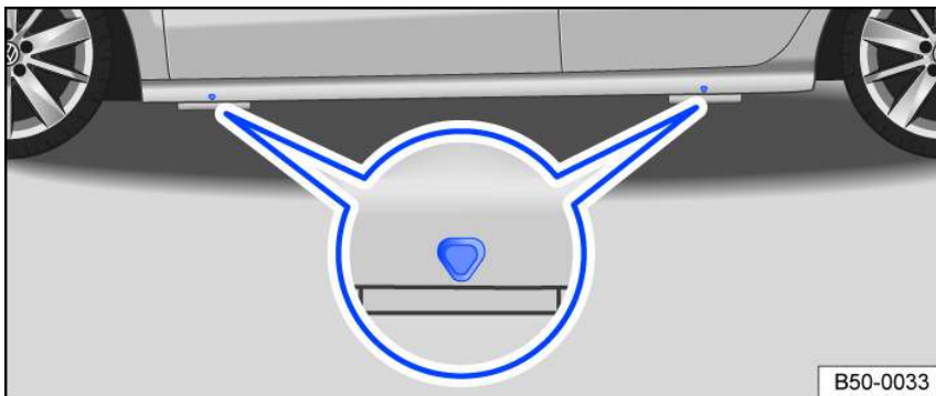
Fig. 158 Lift points for the vehicle jack (general example).
