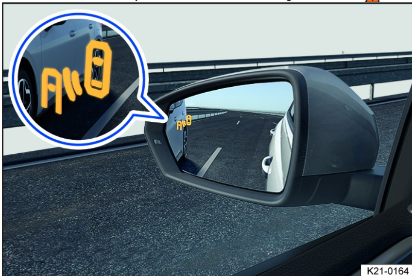
Fig. 104 In the outside mirrors: Blind Spot Monitor indicator.
