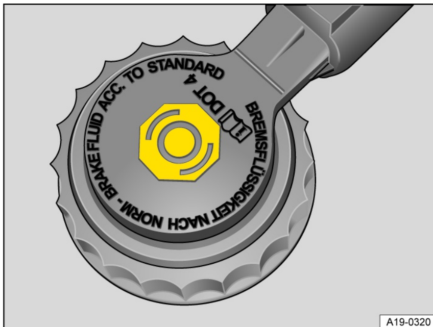
Fig. 144 In the engine compartment: cap on the brake fluid reservoir (version 1).
