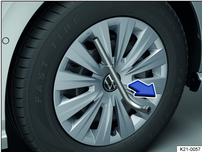
Fig. 153 Remove the wheel hub cover.
