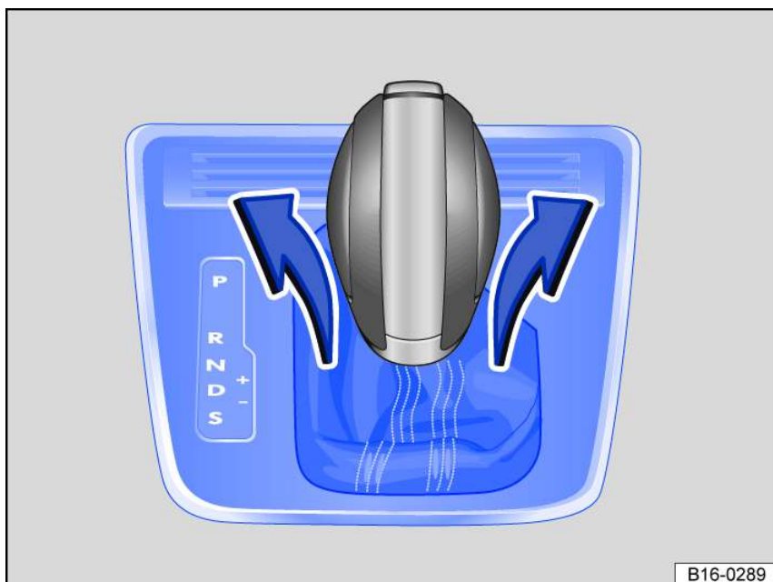
Fig. 93 Remove the cover on the shift gate.
