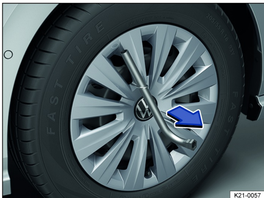
Fig. 166 Remove the wheel hub cover.
