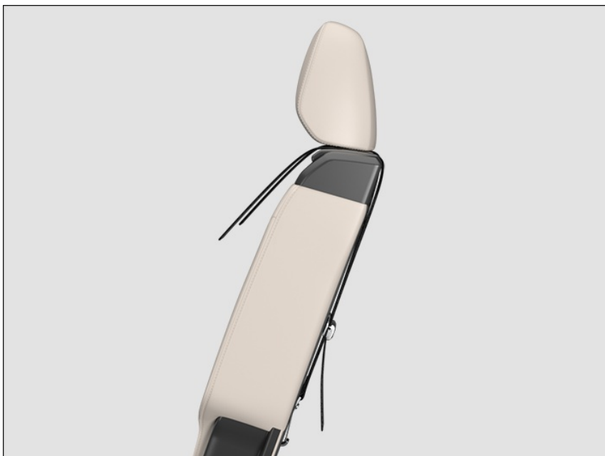
Fig. 36 On the rear side of the outer seats of the second row of seats: Attached top tether safety belt.
