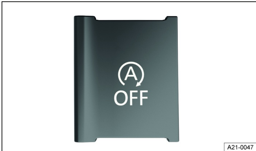
Fig. 90 In the lower section of the center console or, depending on the vehicle equipment, in the Infotainment system: Button for the start-stop system.
