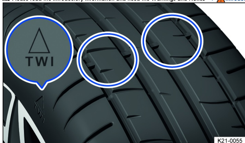
Fig. 163 Tire tread: tread wear indicator.
