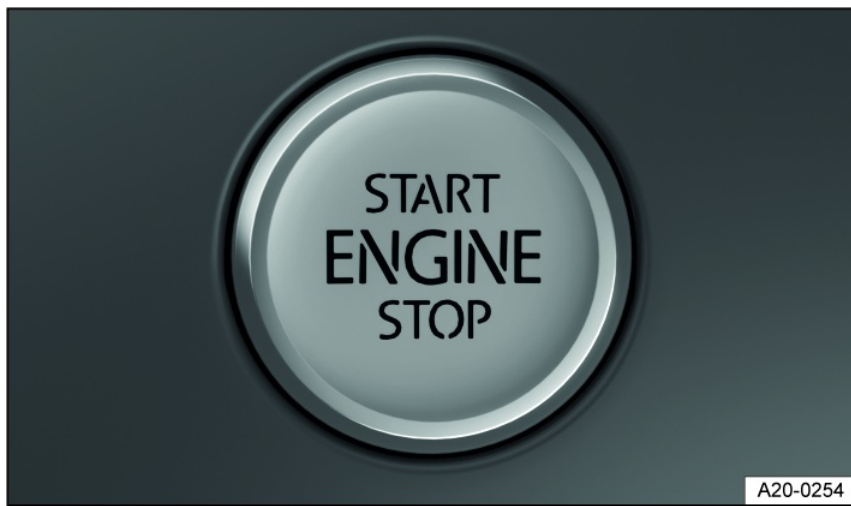
Fig. 87 In the lower area of the center console: starter button for starting the engine.
