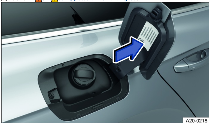
Fig. 129 On the inside of the fuel filler flap: fuel label (general example)
