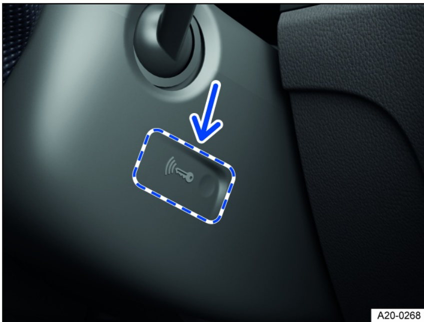
Fig. 89 On the right side of the steering column: emergency start function.
