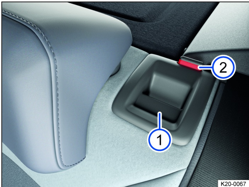
Fig. 64 In the rear seat backrest: release button.
