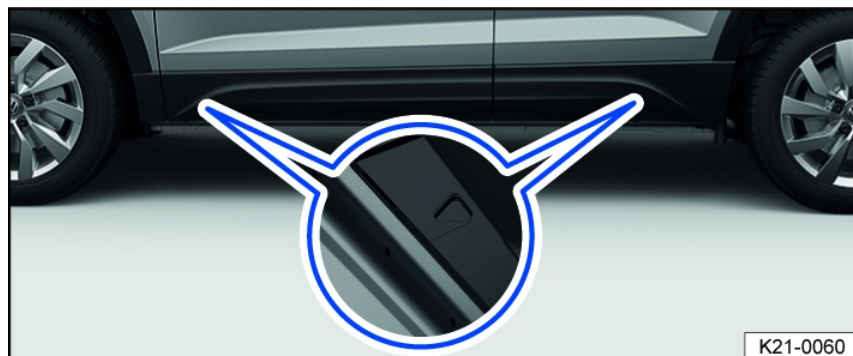
Fig. 173 Mounting points for the vehicle jack.
