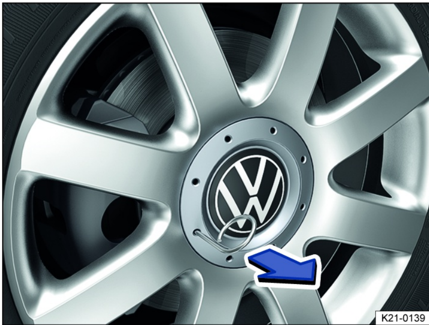
Fig. 165 Remove the hubcap.
