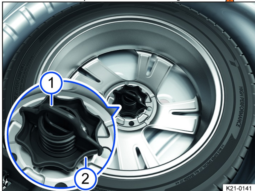
Fig. 172 In the luggage compartment: handle to secure the compact spare wheel.
