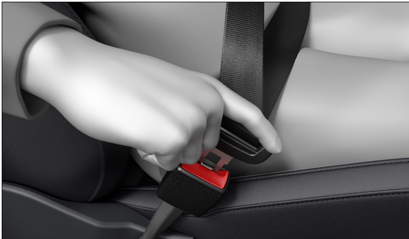
Fig. 21 Inserting the buckle tongue into the safety belt buckle.
