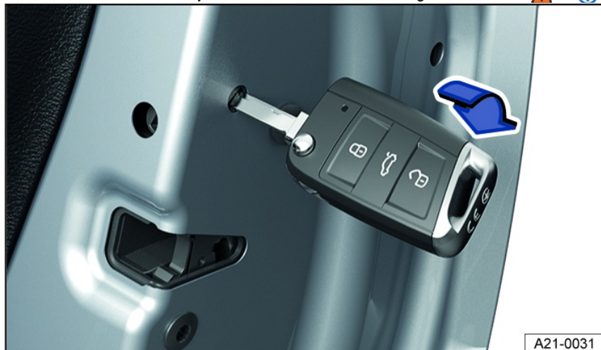
Fig. 50 In the front edge of the rear right-hand door: Vehicle emergency lock for using the emergency key (variant 1).
