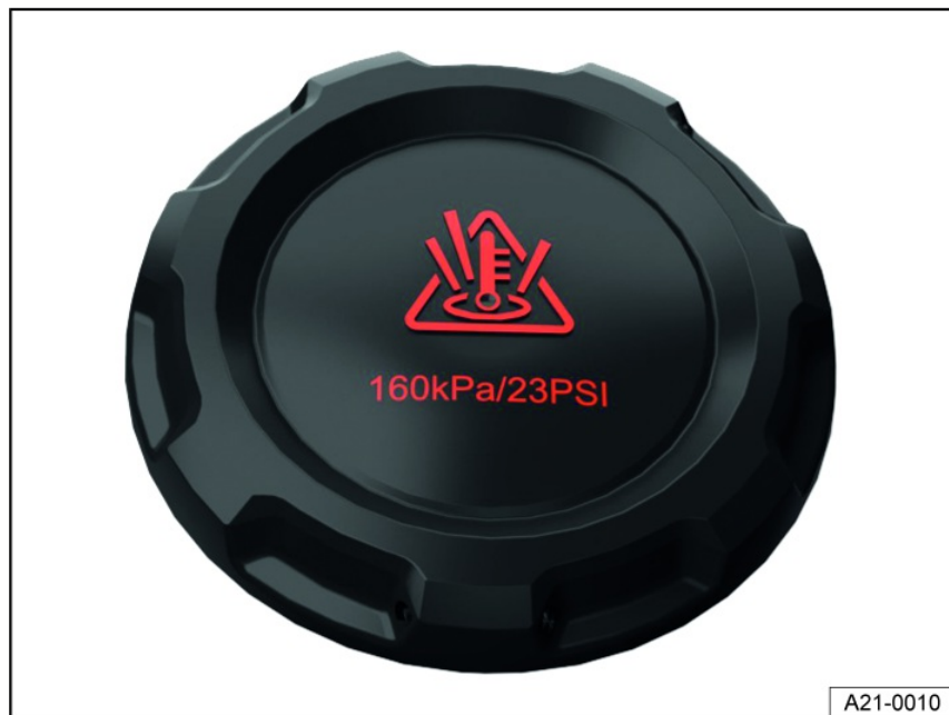
Fig. 156 In the engine compartment: cap on the engine coolant expansion tank.
