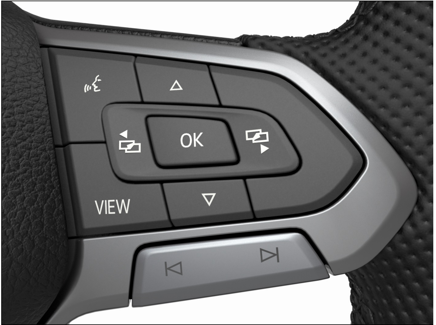
Fig. 12 Right side of the multi-function steering wheel: buttons for operating the menus and information displays in the Volkswagen Digital Cockpit Basic Version.
