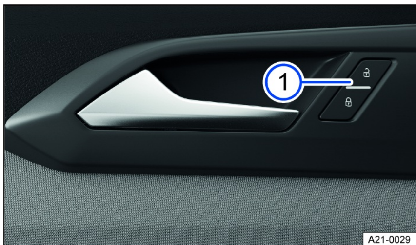
Fig. 48 In the driver's door: central locking button.
