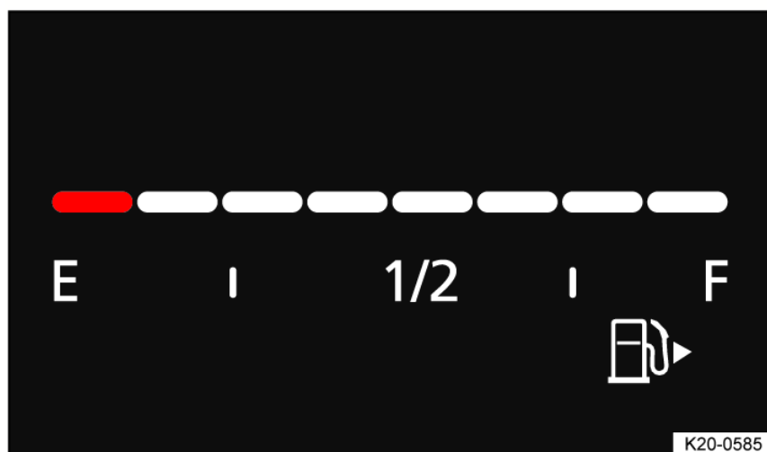
Fig. 14 Fuel gauge on the Volkswagen Digital Cockpit Basic version (general example).
