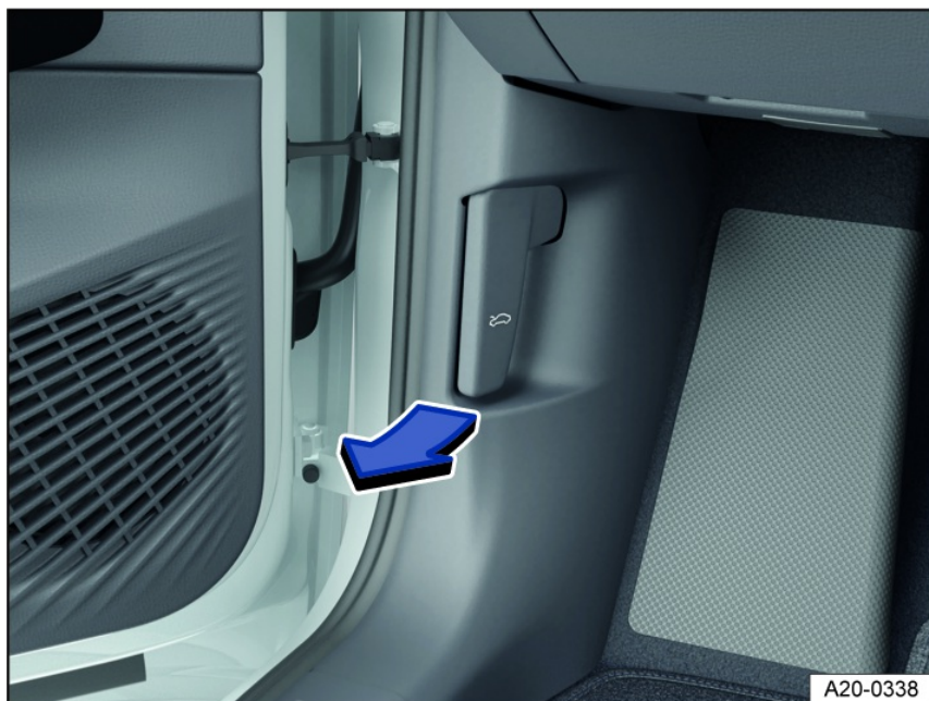
Fig. 148 In the driver's side footwell: Release lever for the hood (general example).
