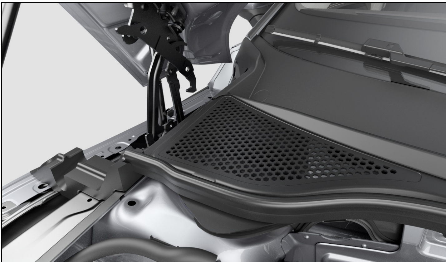
Fig. 177 Between the engine compartment and windshield: plenum chamber (general example).
