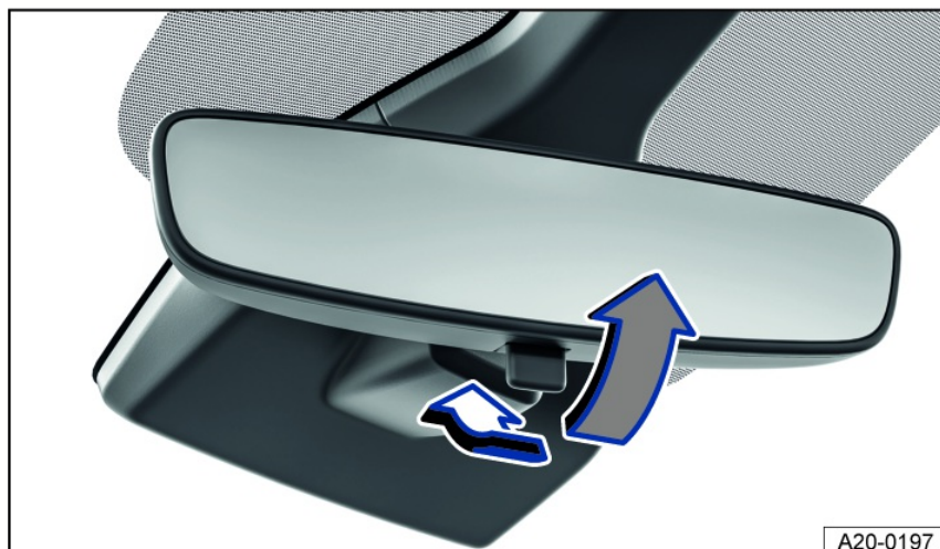
Fig. 79 On the windshield: manual dimming interior rearview mirror.
