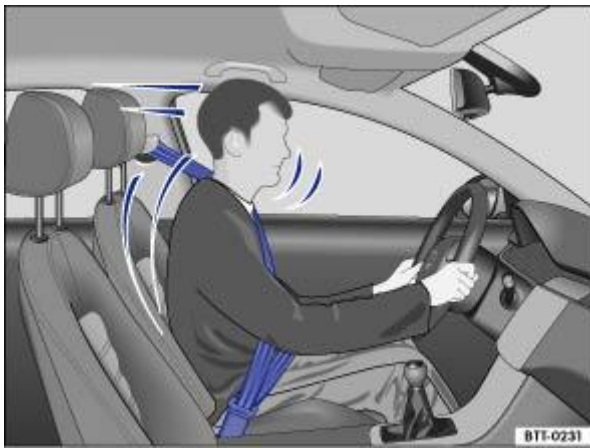
Fig. 33 Driver restrained by a properly worn seat belt during a sudden braking manoeuvre.
