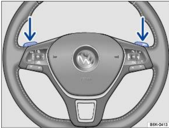
Fig. 107 Steering wheel with paddles for Tiptronic.
