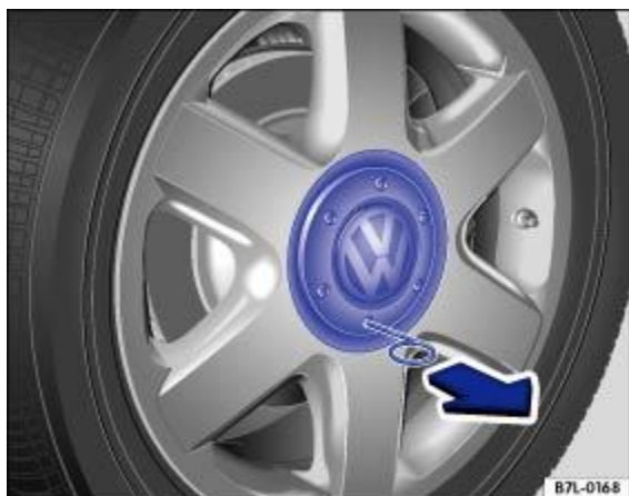
Fig. 199 Removing the centre wheel trim by pulling.
