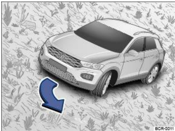
Fig. 115 Steering into the fall line.
