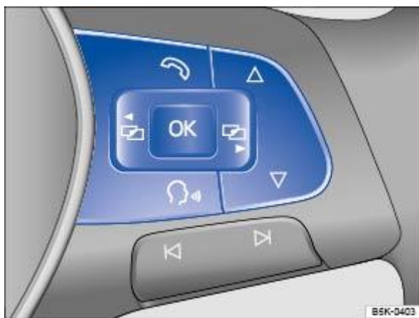
Fig. 21 Right-hand side of the multifunction steering wheel: controls for using the menus and information displays in the instrument cluster.
