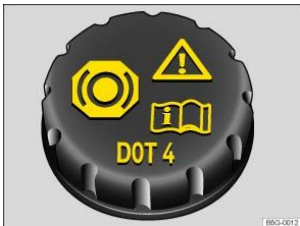
Fig. 190 In the engine compartment: cap on the brake fluid reservoir.
