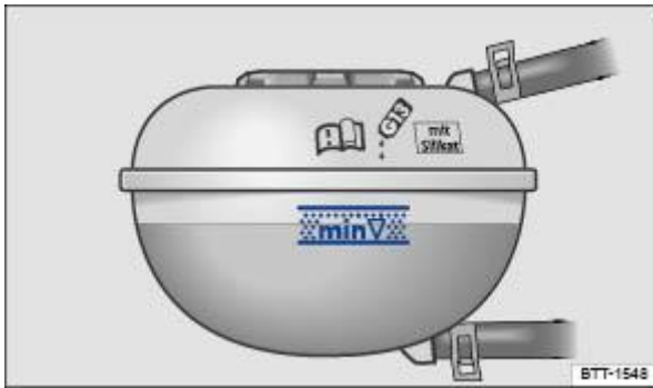
Fig. 188 In the engine compartment: markings on the coolant expansion tank.
