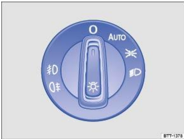
Fig. 79 Next to the steering wheel: light switch (one variant).
