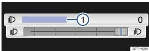
Fig. 82 In the Infotainment system: slider for headlight range control.
