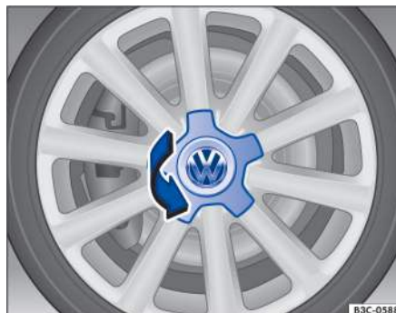
Fig. 182 Twisting the hubcap off.
