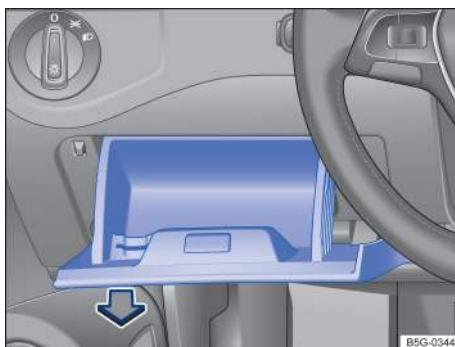
Fig. 156 On the driver side in the instrument panel: Removing the storage compartment to access fuses.
