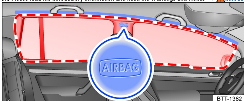
Fig. 38 On the left side of the vehicle: installation location and deployment zone of the Side Curtain Protection®.
