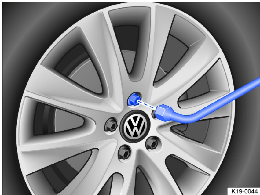
Fig. 179 Wheel change: removing wheel bolts with the lug wrench.
