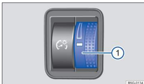
Fig. 79 To the left of the steering wheel: Thumbwheel to adjust instrument panel lighting ①.
