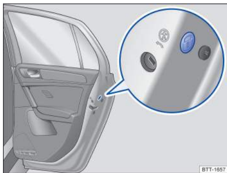
Fig. 55 On the front side of the rear passenger door: Manual lock, covered by a rubber seal.
