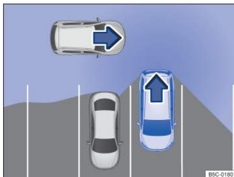
Fig. 123 Rear Traffic Alert: Monitored area around the vehicle that is backing out of a parking space.
