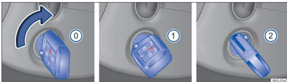
Fig. 96 In the ignition switch: Vehicle key positions for vehicles without Keyless Access.
