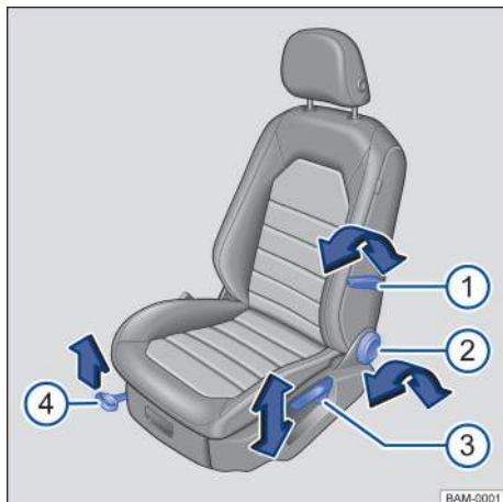
Fig. 68 Driver seat: Manual seat adjustment controls.
