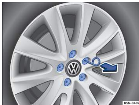
Fig. 184 Pulling cover caps off wheel bolts.
