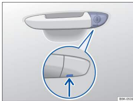
Fig. 53 Driver door: Concealed lock cylinder.
