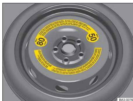
Fig. 179 In the luggage compartment: Compact spare wheel (label design may vary).
