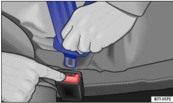
Fig. 35 Removing the latch plate from the buckle.
