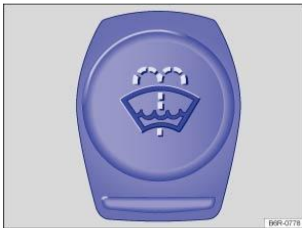
Fig. 185 In the engine compartment: cap on the washer fluid reservoir.
