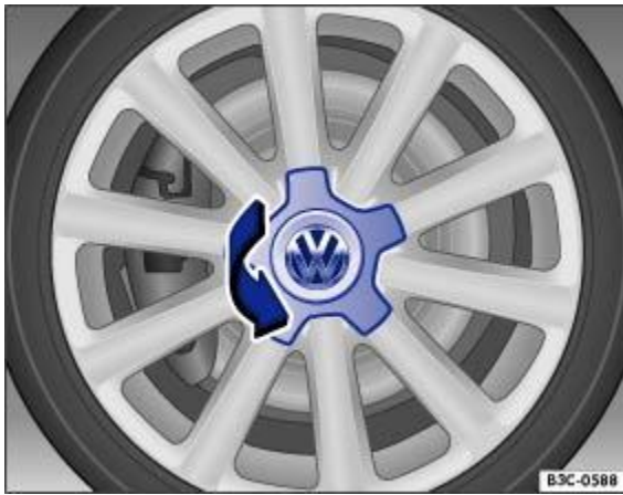
Fig. 200 Removing the centre wheel trim by turning.
