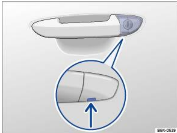
Fig. 56 Driver door handle: concealed lock cylinder.
