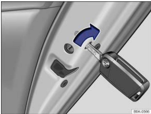
Fig. 58 In the front edge of the rear right-hand door: manually locking the vehicle with the vehicle key.
