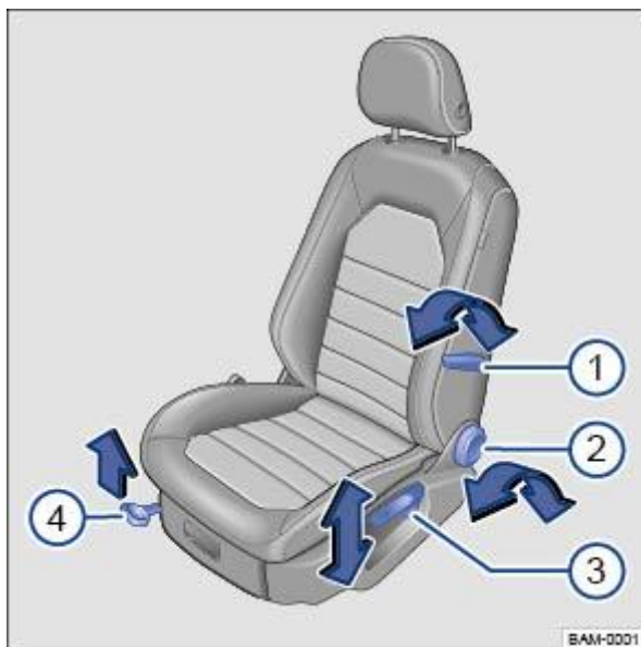
Fig. 69 On the left front seat: controls.
