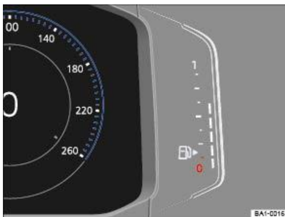
Fig. 16 Fuel gauge in the Active Info Display.
