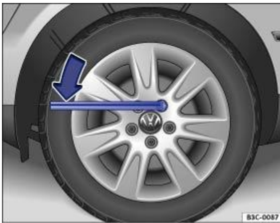
Fig. 203 Changing a wheel: loosening the wheel bolts.
