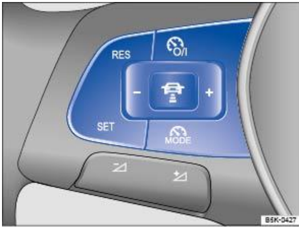
Fig. 117 Left-hand side of the multifunction steering wheel: buttons for operating the speed limiter.
