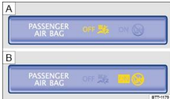
Fig. 39 In the roof console: indicator lamp for deactivated front passenger front airbag or indicator lamp for activated front passenger front airbag .
