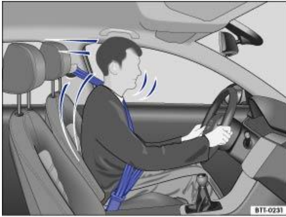
Fig. 33 Driver restrained by a properly worn seat belt during a sudden braking manoeuvre.
