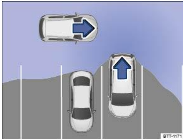
Fig. 133 Illustration of Rear Traffic Alert: monitored area around the vehicle leaving the parking space.
