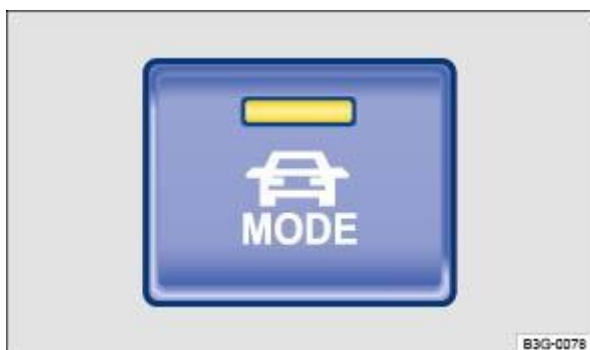
Fig. 110 In the lower section of the centre console: driving profile selection button.
