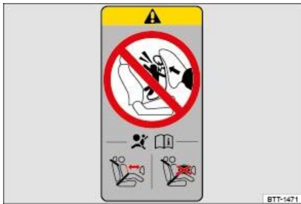
Fig. 45 Illustration: airbag label on the B-pillar.
