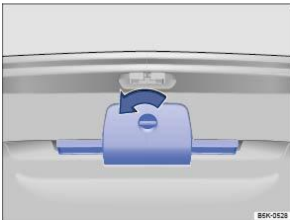
Fig. 48 In the boot lid: holder for the warning triangle.
