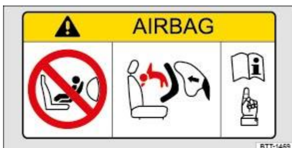
Fig. 44 Illustration: airbag label on the sun visor.
