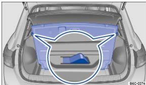
Fig. 148 In the luggage compartment: locking the luggage compartment floor.
