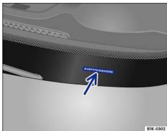
Fig. 216 Vehicle identification number.
