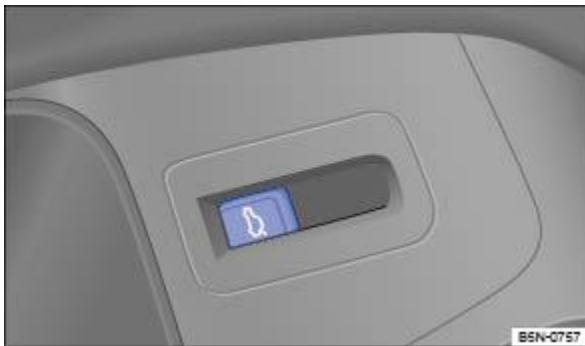
Fig. 55 In the driver door: release for the boot lid.
