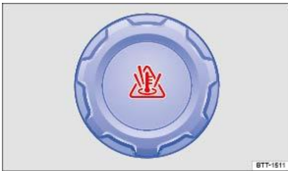
Fig. 189 In the engine compartment: coolant expansion tank cap (illustration).
