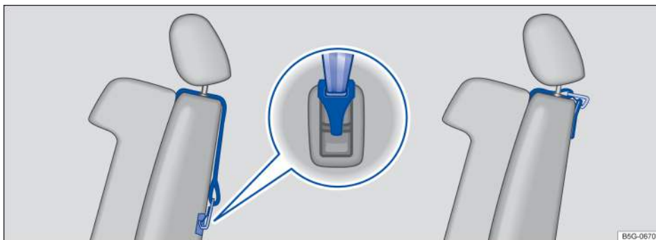
Fig. 45 Example of a mounted upper tether strap: The version on the left shows an outer seating position. The version on the right shows the center seating position.
