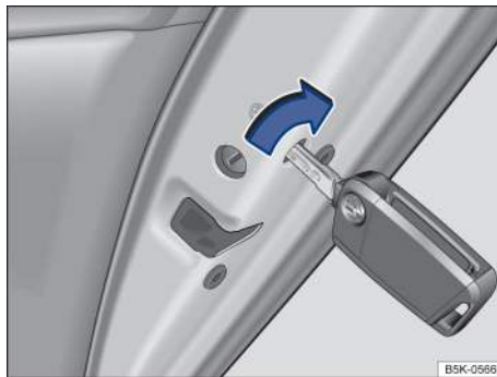
Fig. 56 On the front side of the rear passenger door: Locking the vehicle with the key bit in the vehicle key.
