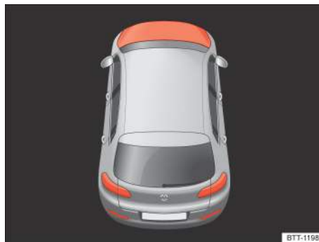
Fig. 168 In the instrument cluster display: Engine hood open or not properly closed.
