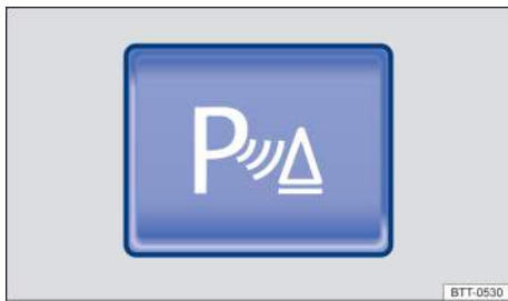
Fig. 116 In the lower center console: Button to switch the Park Distance Control system on or off.
