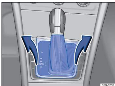
Fig. 104 Removing the selector gate cover.
