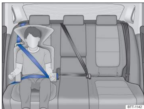
Fig. 42 Child properly restrained in a booster seat on the rear seat.
