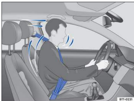
Fig. 27 Belted driver secured by the correctly worn safety belt in the event of a sudden braking maneuver.
