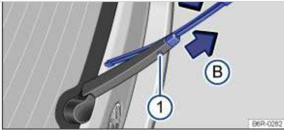
Fig. 205 Changing the rear window wiper blades.
