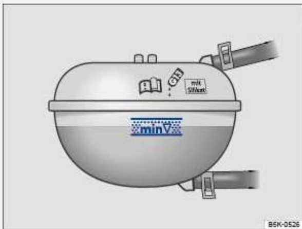
Fig. 201 Coolant expansion tank in the engine compartment.
