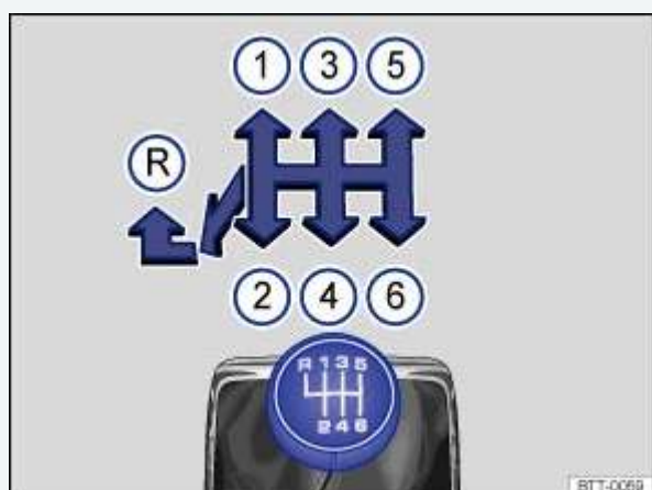
Fig. 140 Gearshift pattern of a 6-speed manual transmission.
