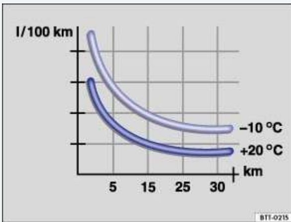
Fig. 150 Fuel consumption in l/100 km at 2 different outside air temperatures.
