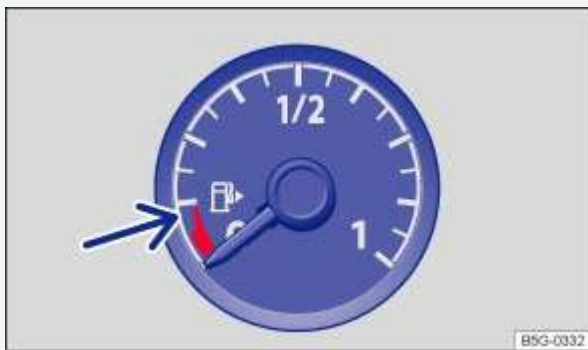
Fig. 194 In the instrument cluster: Fuel gauge.
