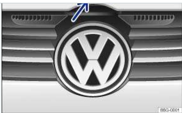
Fig. 197 Above the radiator grille: Outside engine hood release.
