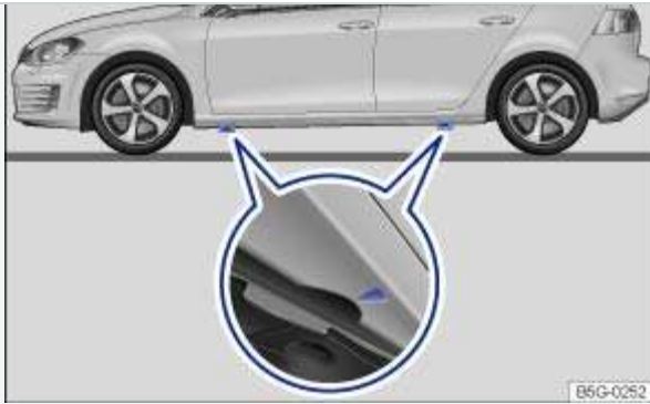
Fig. 226 Lift points for the jack.
