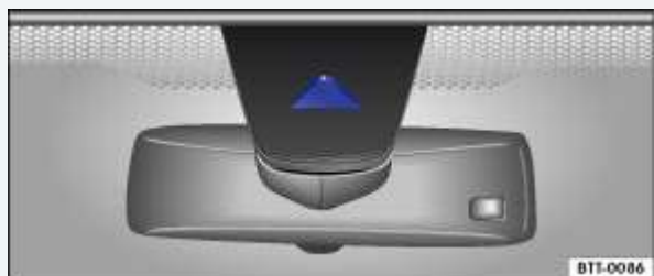
Fig. 168 In the front windshield: Area of the Lane Assist camera.
