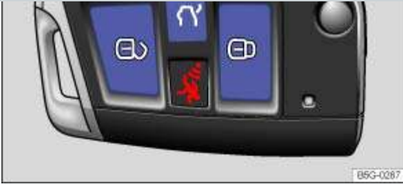
Fig. 28 Remote control vehicle key with panic button.
