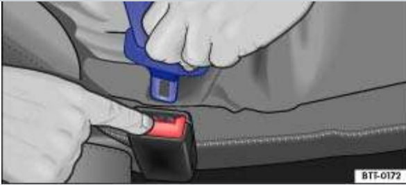
Fig. 63 Releasing the buckle tongue from the belt buckle.
