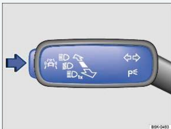
Fig. 18 On the turn signal and high beam lever: Driver assistance systems button.
