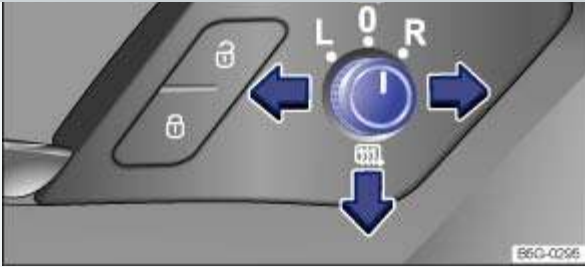
Fig. 98 In the driver door: Adjusting knob for the outside mirrors.
