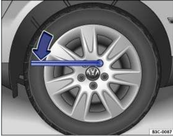
Fig. 222 Changing a wheel: Loosening the wheel bolts.
