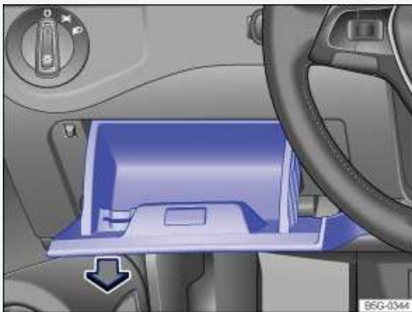
Fig. 231 On the driver side in the instrument panel: Fuse box cover.
