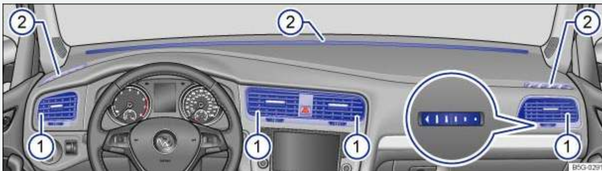
Fig. 193 In the instrument panel: Air vents.
