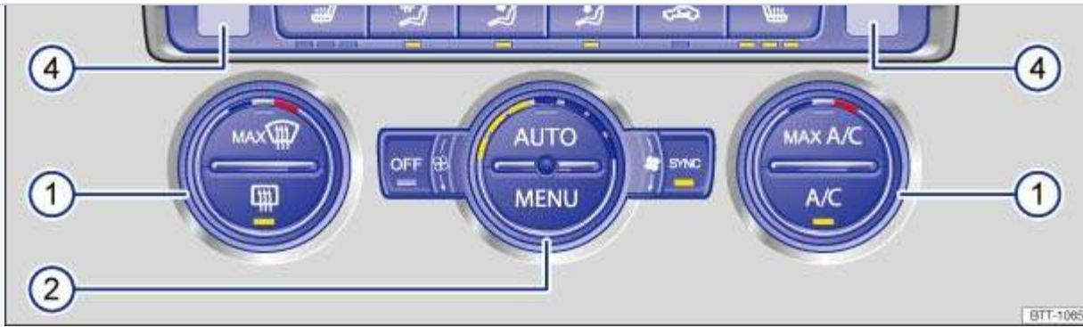
Fig. 192 In the center console: Climatronic controls.
