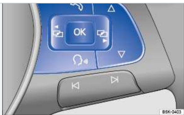
Fig. 17 Right side of the multi-function steering wheel (if equipped): Controls for the menus and information in the instrument cluster display.
