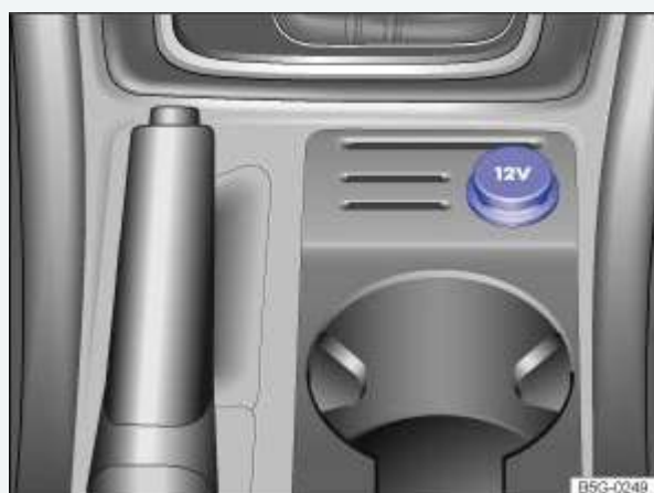
Fig. 132 In the lower center console: 12 Volt socket (vehicles with parking brake lever).
