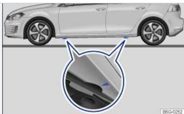
Fig. 226 Lift points for the jack.
