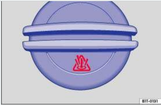
Fig. 202 Coolant expansion tank cap in the engine compartment.
