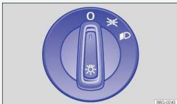
Fig. 85 Headlight switch next to the steering wheel.
