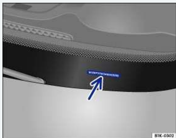
Fig. 24 Vehicle identification number (VIN).
