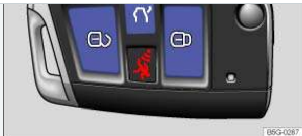
Fig. 28 Remote control vehicle key with panic button.
