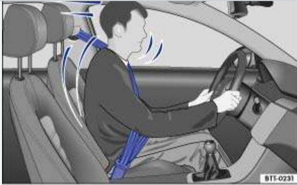
Fig. 61 Belted driver secured by the correctly worn safety belt in the event of a sudden braking maneuver.
