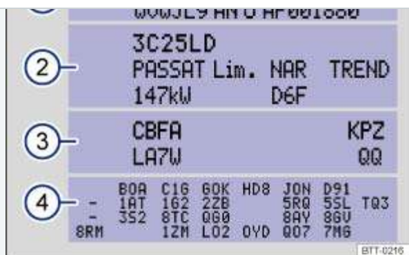
Fig. 23 Vehicle identification label: Shown in the example with engine identification code CBFA ③.
