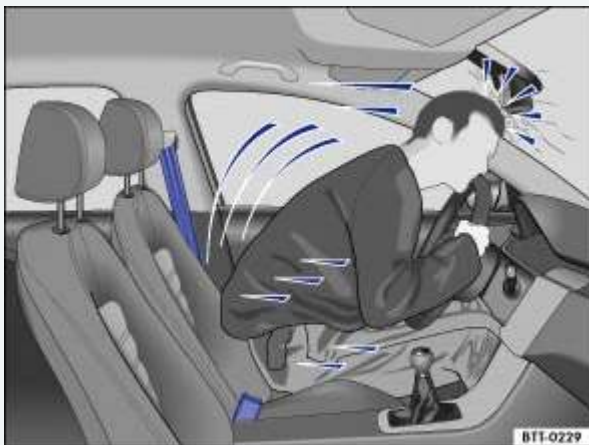
Fig. 59 The unbelted driver is thrown forward.
