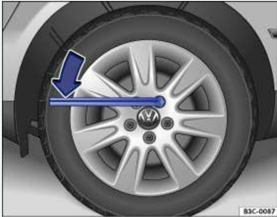
Fig. 222 Changing a wheel: Loosening the wheel bolts.
