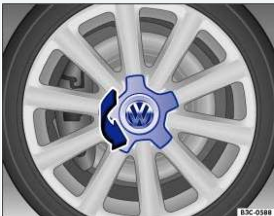
Fig. 218 Pulling the hubcap off.
