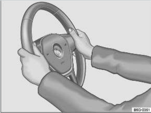
Fig. 50 Steering wheel: 9 o'clock and 3 o'clock positions.
