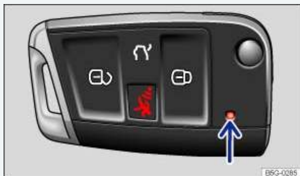
Fig. 26 Indicator light in the remote control vehicle key.
