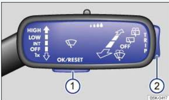
Fig. 16 On the right side of the steering column (vehicles without a multi-function steering wheel): Windshield wiper lever with controls for instrument cluster menus and displays.
