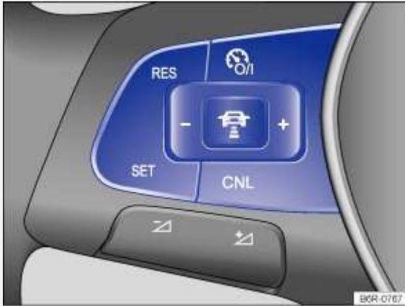
Fig. 160 Left-hand side of the multifunction steering wheel: Buttons for operating the Adaptive Cruise Control (ACC).
