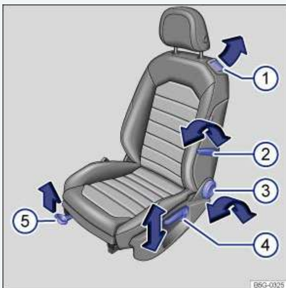
Fig. 41 Driver seat: Manual seat adjustment controls.
