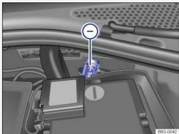
Fig. 235 In the engine compartment: Negative jump-start terminal ⊖.
