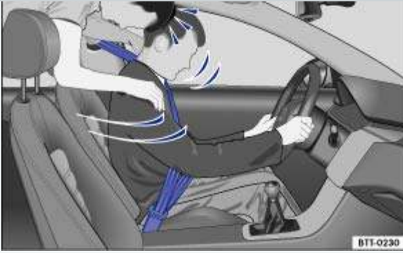
Fig. 60 Unbelted passengers in the rear seats are thrown forward on top of the belted driver.
