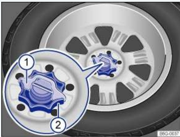
Fig. 114 In the luggage compartment: Handwheel holding the spare wheel in place (if equipped).
