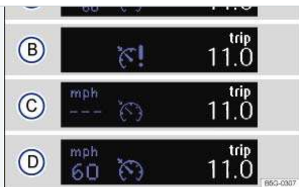
Fig. 153 In the instrument cluster display: Cruise control status indications.
