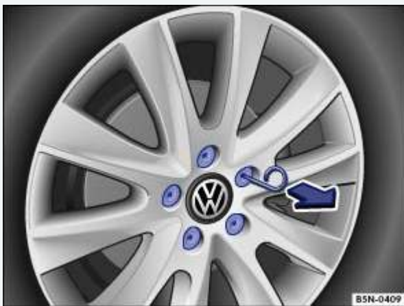
Fig. 220 Pulling cover caps off wheel bolts.
