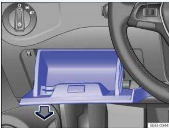
Fig. 231 On the driver side in the instrument panel: Fuse box cover.
