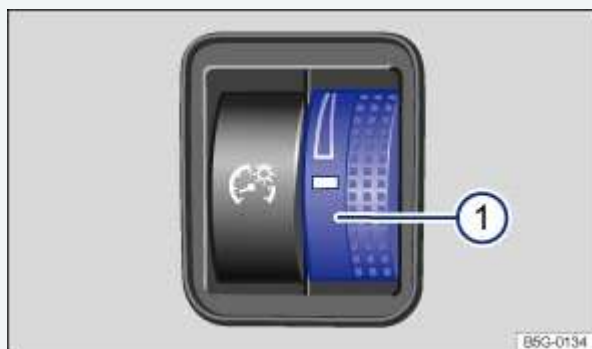
Fig. 87 To the left of the steering wheel: Thumbwheel to adjust instrument panel lighting ①.
