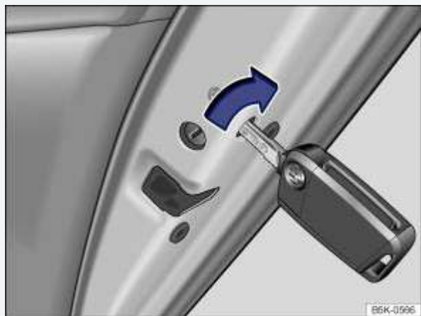
Fig. 211 On the front side of the passenger side rear door: Locking the vehicle with the key bit in the vehicle key.
