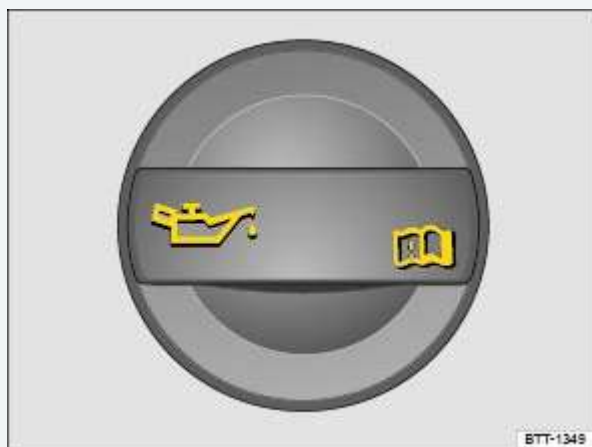
Fig. 199 In the engine compartment: Engine oil filler cap (cap design may vary depending on vehicle equipment).
