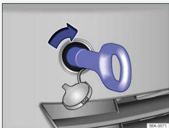
Fig. 238 In the right front bumper: Installing the towing eye.
