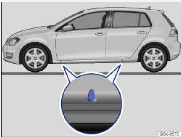
Fig. 224 Lift points for the jack.
