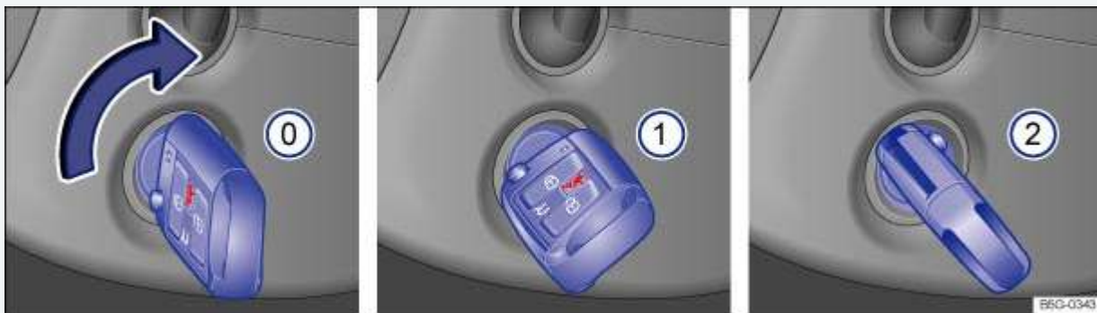
Fig. 134 In the ignition switch: Vehicle key positions.
