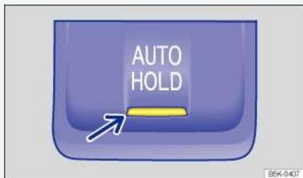
Fig. 152 In the lower center console: Button for Auto Hold (if equipped).
