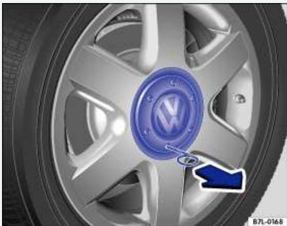
Fig. 218 Pulling the hubcap off.
