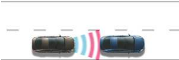
Depiction of Forward Collision Warning and Autonomous Emergency Braking (Front Assist)
