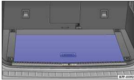
Fig. 261 Location of the high-voltage battery: under the luggage compartment floor.
