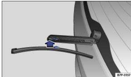
Fig. 322 Changing the rear window wiper blades.
