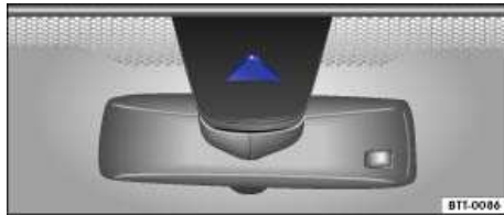
Fig. 279 In the front windshield: Area of the Lane Assist camera.
