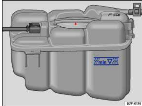
Fig. 319 Coolant expansion tank in the engine compartment.
