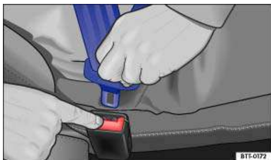
Fig. 55 Removing the latch plate from the buckle
