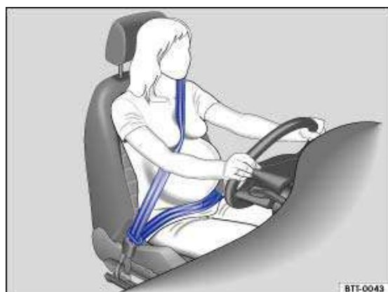
Fig. 57 Correct seat belt routing during pregnancy
