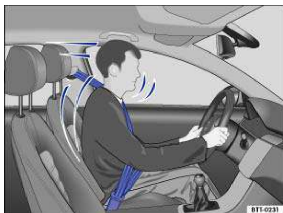
Fig. 53 Driver restrained by a properly positioned seat belt during a sudden braking manoeuvre
