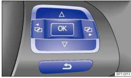
Fig. 17 Right side of the multi-function steering wheel (if equipped): Controls for the menus in the instrument cluster.
