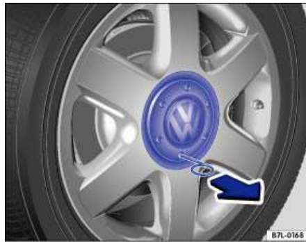
Fig. 160 Pulling the hubcap off.
