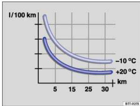
Fig. 125 Fuel consumption in l/100 km at 2 different outside air temperatures.
