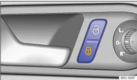
Fig. 26 In the vehicle doors: Power locking button.
