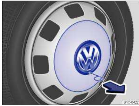
Fig. 164 Pulling the wheel cover off (Version 2).
