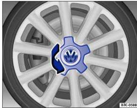
Fig. 161 Twisting the hubcap off.
