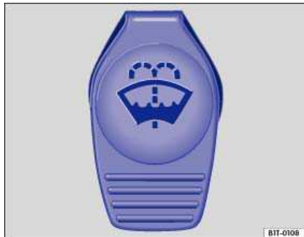
Fig. 82 In the engine compartment: Cap of the windshield washer fluid reservoir.
