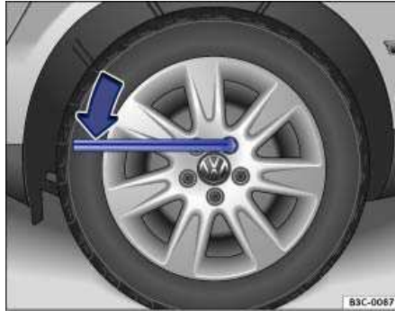
Fig. 165 Changing a wheel: Loosening the wheel bolts.
