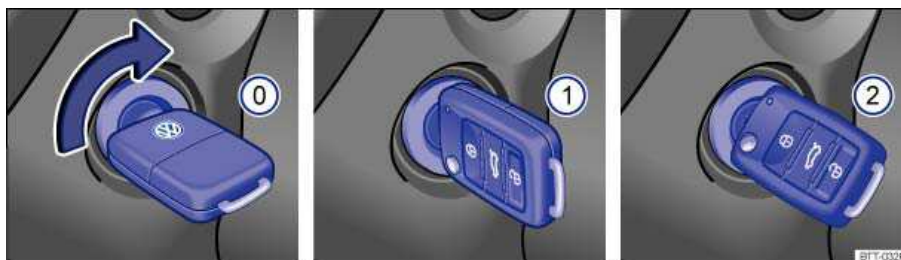
Fig. 111 In the ignition switch: Vehicle key positions.
