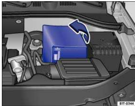
Fig. 146 In the engine compartment: Open the sleeve covering of the vehicle battery.
