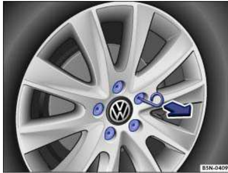
Fig. 162 Pulling cover caps off wheel bolts.
