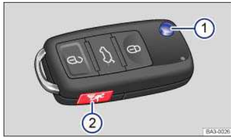
Fig. 21 Remote control vehicle key with panic button.
