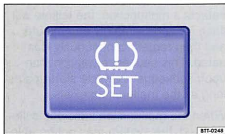
Fig. 120 In the glove compartment: SET button for the Tire Pressure Monitoring System.
