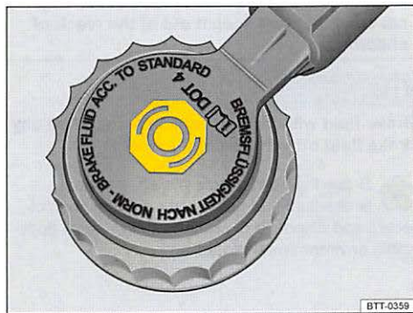
Fig. 115 In the engine compartment: Brake fluid reservoir cap.
