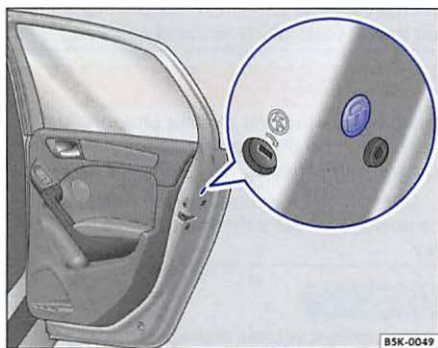
Fig. 147 On the front side of the right rear door: Emergency lock, covered by a rubber seal.
