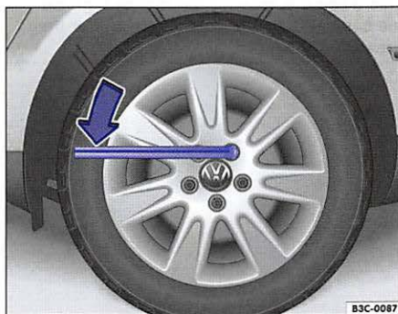
Fig. 160 Changing a wheel: Loosening wheel bolts.
