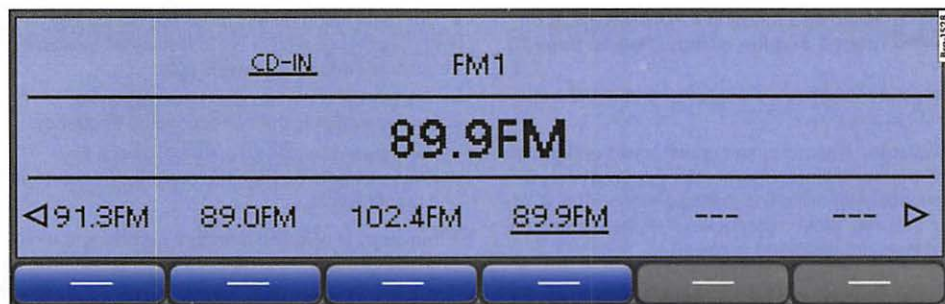
Fig. 5 Changing stations using the [◀ SEEK / ... ▶] rocker switch is only possible for preset stations.
