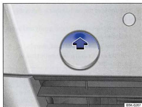
Fig. 202 In right front bumper: Remove cover.
