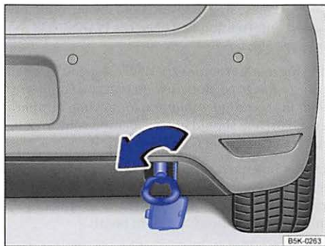
Fig. 205 On the right in the rear bumper: Screwed-in towing eye.
