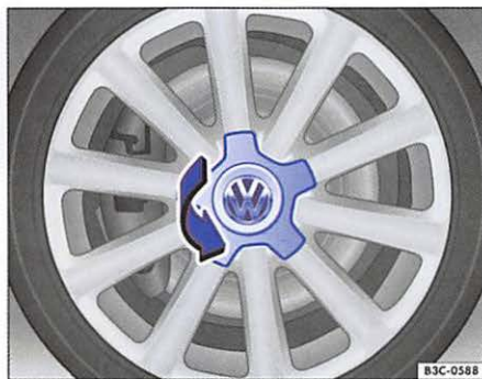
Fig. 179 Twisting off hubcap.
