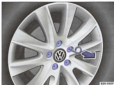
Fig. 181 Pulling cover caps off wheel bolts.
