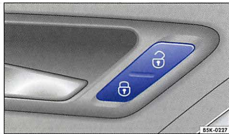
Fig. 18 In the driver door: power locking switch.
