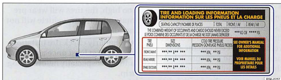
Fig. 161 Location of the tire inflation pressure label.
