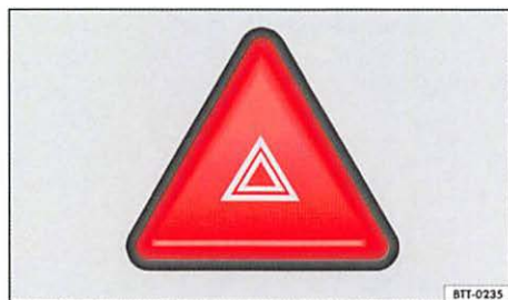
Fig. 167 In the center of the instrument panel: Switch for emergency flashers.
