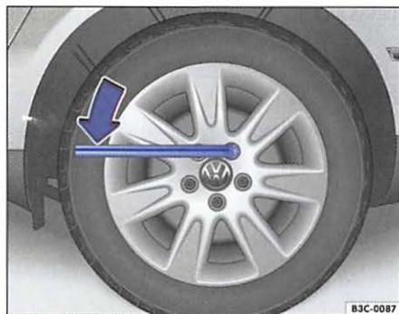
Fig. 182 Changing a wheel: Loosening wheel bolts.
