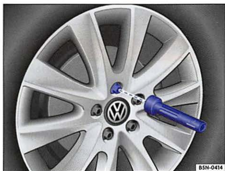
Fig. 186 Changing a wheel: remove previously loosened wheel bolts using the screwdriver handle.
