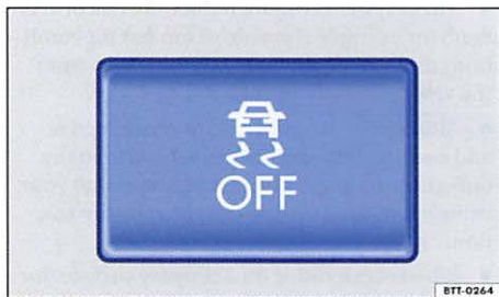
Fig. 128 In the center console: Button to manually switch ASR function on and off (vehicles with ESP).
