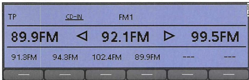
Fig. 4 Changing stations using the [◀ SEEK / ... ▶] rocker switch.
