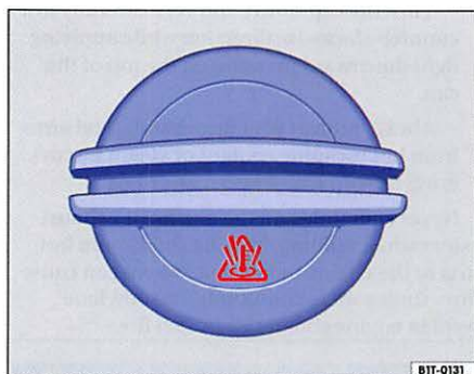
Fig. 155 Coolant expansion tank cap in the engine compartment.
