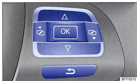
Fig. 9 Right side of the multi-function steering wheel: Controls for the menus in the instrument cluster.
