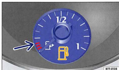
Fig. 147 In the instrument cluster: fuel gauge. ▶
