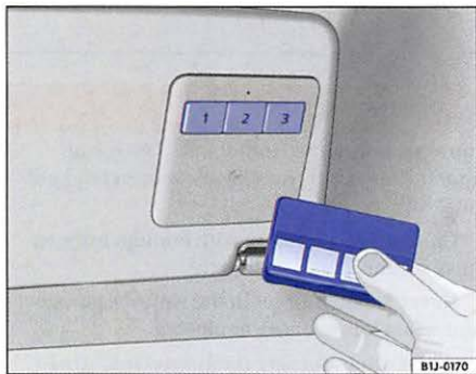
Fig. 28 The remote control and buttons for the HomeLink Universal Transmitter are in the sun visor.
