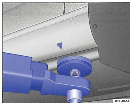
Fig. 165 Front lift point for workshop hoist or floor jack.
