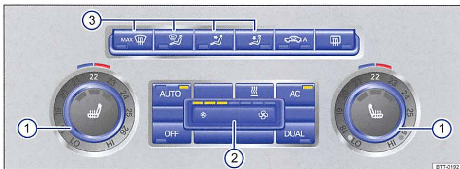
Fig. 144 In the center console: Climatronic controls.
