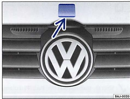
Fig. 150 Secondary hood release in the radiator grille.
