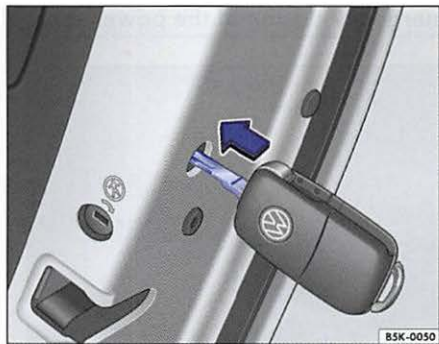
Fig. 170 Using the vehicle key to lock the vehicle.
