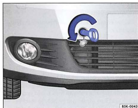
Fig. 203 In right front bumper: Screwing in towing eye.
