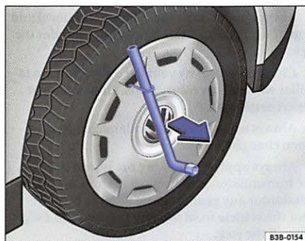
Fig. 180 Pulling the wheel cover off.
