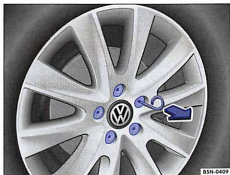
Fig. 159 Pulling cover caps off wheel bolts.
