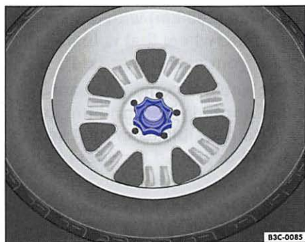
Fig. 140 In the luggage compartment: Hand wheel holding spare wheel in place.
