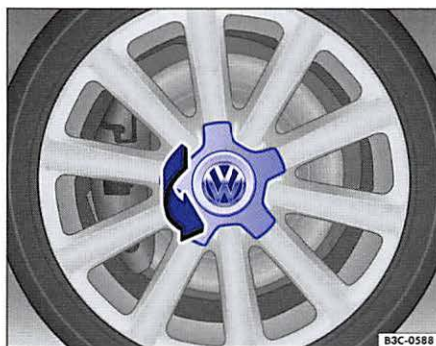
Fig. 157 Twisting off the hubcap.
