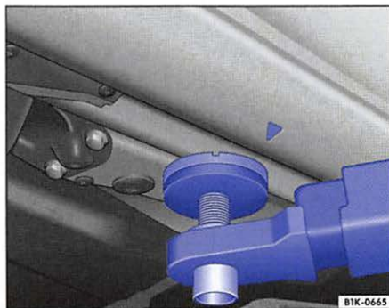
Fig. 144 Rear lift point for workshop hoist or floor jack.
