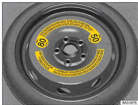
Fig. 141 In the luggage compartment: Hand wheel holding compact spare wheel in place.
