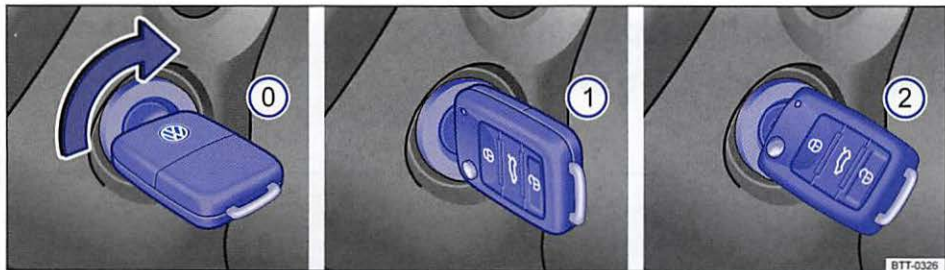
Fig. 104 In the ignition switch: Vehicle key positions.
