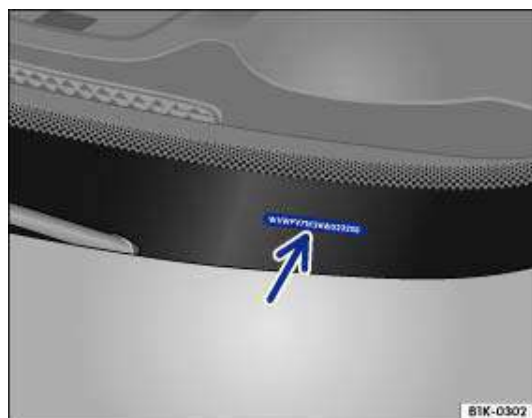
Fig. 20 Vehicle identification number
