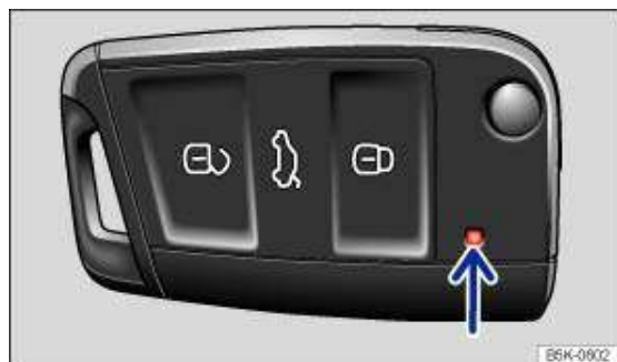
Fig. 23 Indicator lamp in the vehicle key
