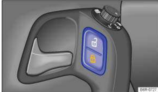
Fig. 28 In the driver door: central locking button
