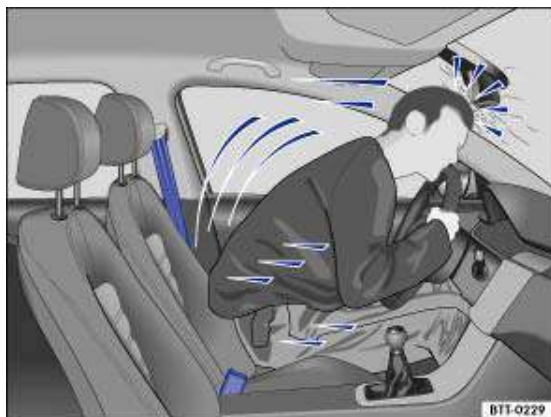
Fig. 51 An unbelted driver is thrown forwards
