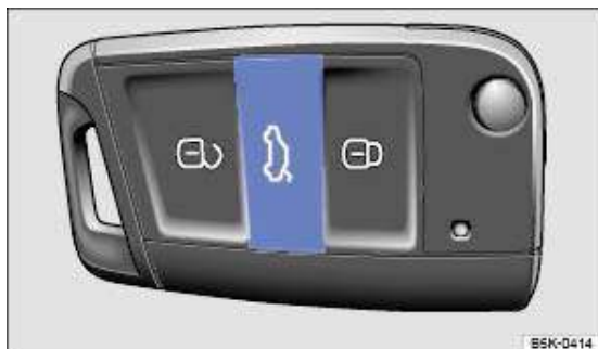
Fig. 33 In the vehicle key: button for unlocking and opening the tailgate
