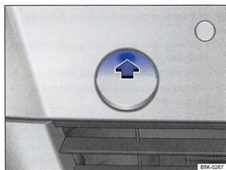
Fig. 202 In right front bumper: Remove cover.
