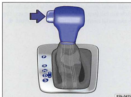
Fig. 124 Automatic transmission selector lever with shift lever release button (arrow).
