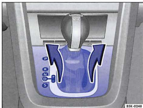
Fig. 152 Removing the selector gate cover.
