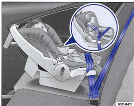
Fig. 65 Rearward-facing infant seat properly installed on the rear seat.
