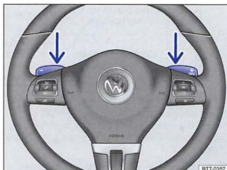
Fig. 112 Steering wheel with optional Tiptronic shift paddles.
