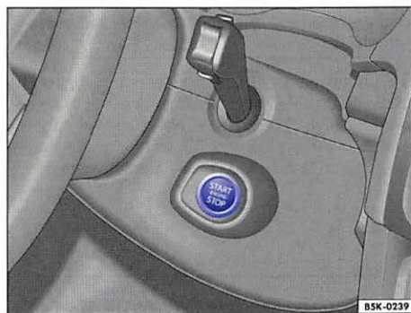
Fig. 105 Keyless Access locking and starting system: Starter button.
