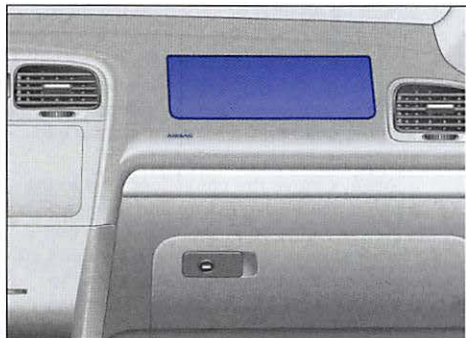
Fig. 60 Location and deployment zone of the passenger front airbag.
