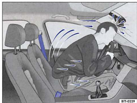
Fig. 48 The unbelted driver is thrown forward.
