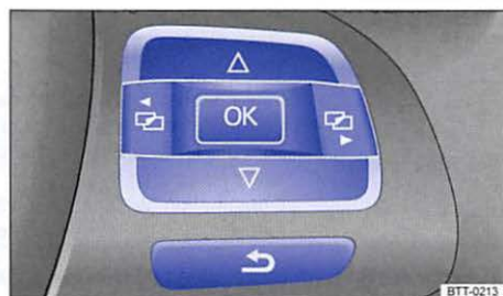
Fig. 13 Right side of the multi-function steering wheel: Controls for the menus in the instrument cluster.
