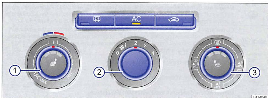
Fig. 121 In the center console: Manual AC controls.
