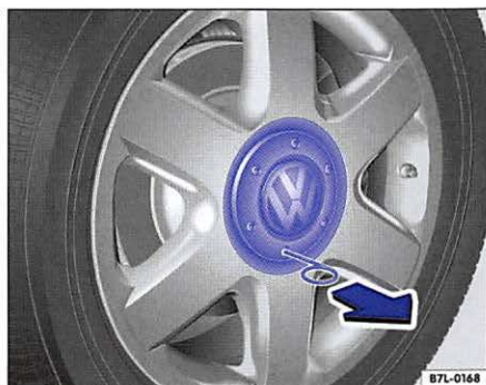
Fig. 156 Pulling off hubcap.
