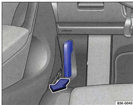
Fig. 126 In the footwell on the driver side: Inside engine hood release lever.
