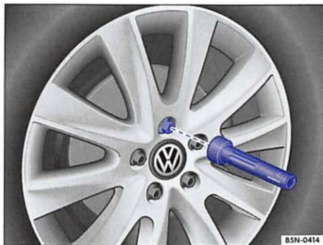
Fig. 164 Changing a wheel: remove previously loosened wheel bolts using the screwdriver handle.
