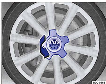
Fig. 157 Twisting off the hubcap.
