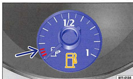
Fig. 124 In the instrument cluster: Fuel gauge.
