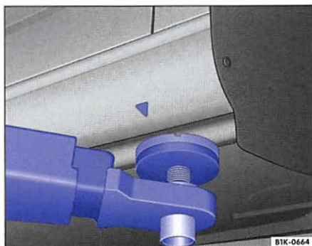
Fig. 143 Front lift point for workshop hoist or floor jack.
