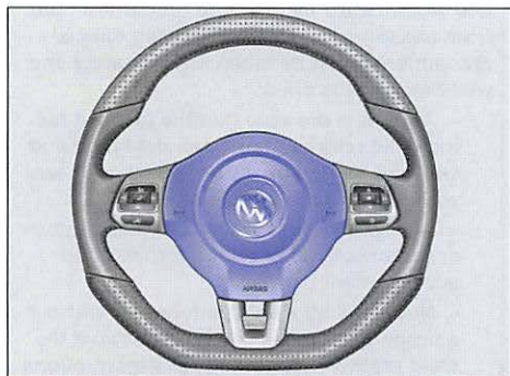
Fig. 59 Location and deployment zone of the driver front airbag.
