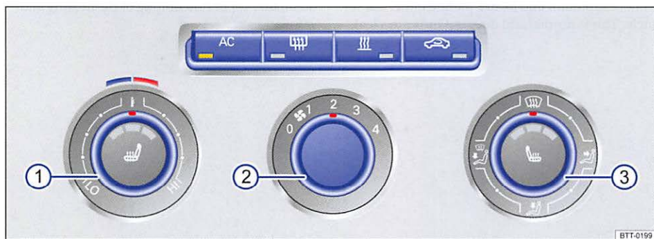
Fig. 143 In the center console: Climatic controls.
