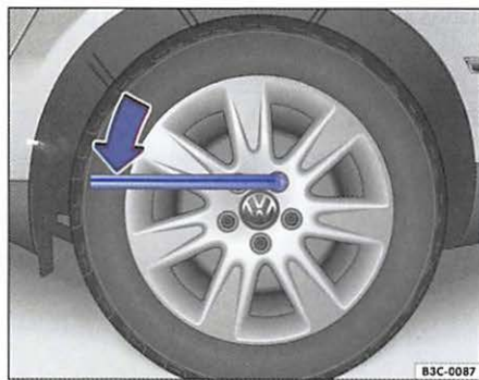
Fig. 182 Changing a wheel: Loosening wheel bolts.
