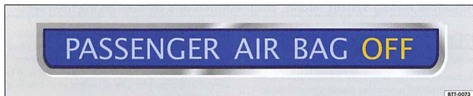
Fig. 57 PASSENGER AIR BAG OFF light on the instrument panel.
