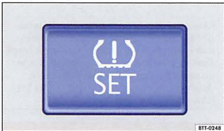
Fig. 142 In the center console or in the glove compartment: Button for the Tire Pressure Monitoring System.
