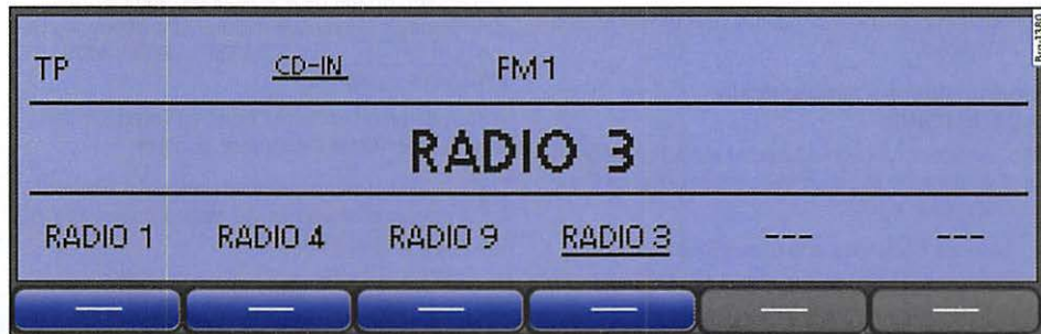
Fig. 9 Displaying station names. TP is switched on and functioning.
