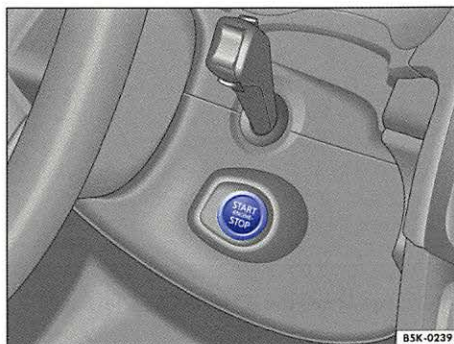
Fig. 119 KESSY locking and starting system: Starter button.
