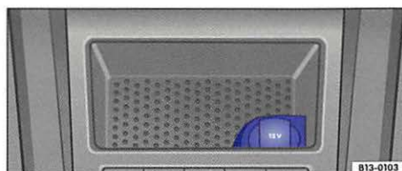
Fig. 116 Front center console: 12 volt socket in the storage compartment.
