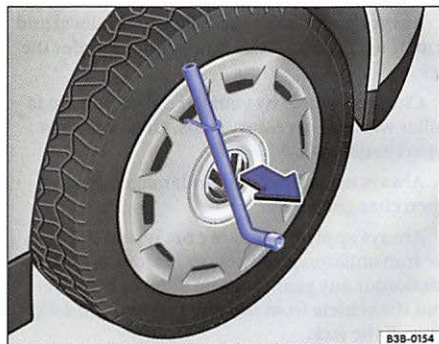
Fig. 180 Pulling the wheel cover off.
