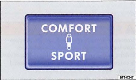
Fig. 141 In the center console: button for Dynamic Chassis Control.
