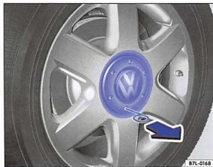
Fig. 178 Pulling off hubcap.
