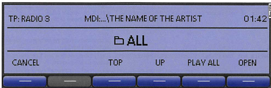
Fig. 24 MEDIA-IN mode: Searches through the folder structure of an MDI source.
