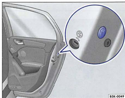
Fig. 169 Emergency lock (covered by a rubber plug) in the edge of the right rear door:
