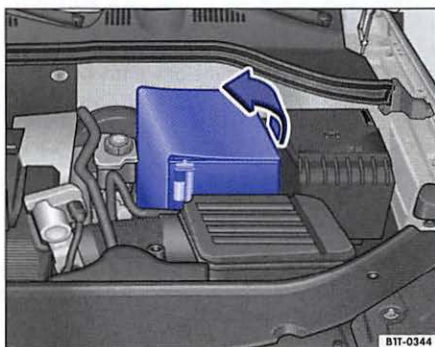
Fig. 134 In the engine compartment: Open the sleeve covering of the vehicle battery.
