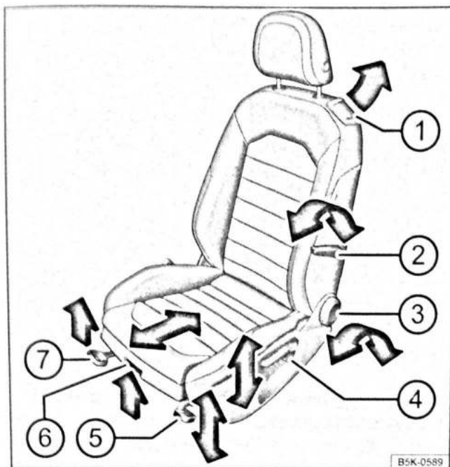
Fig. 43 Front left-hand seat controls
