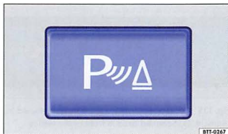
Fig. 132 In the center console: Button to switch the Park Distance Control system ON or OFF.
