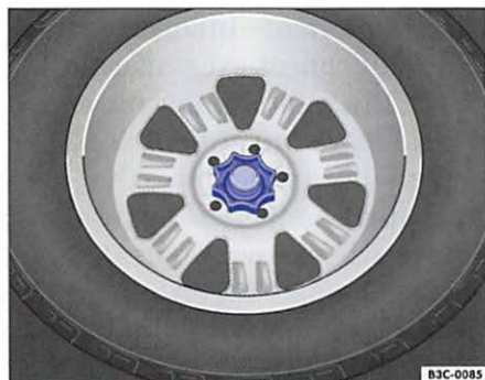
Fig. 163 In the luggage compartment: Hand wheel holding spare wheel in place.
