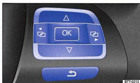
Fig. 3 Buttons on the right side of the multi-function steering wheel.
