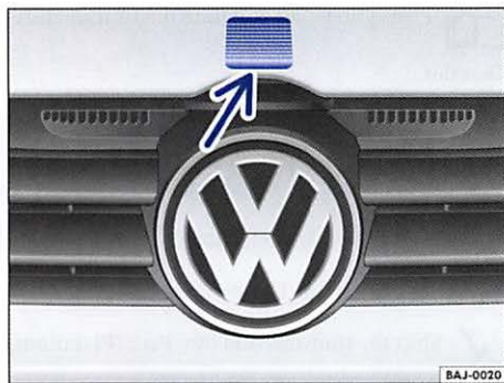
Fig. 150 Secondary hood release in the radiator grille.
