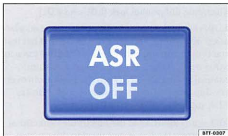
Fig. 129 In the center console: Button to manually switch ASR function on and off (vehicles without ESP).
