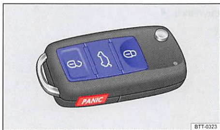
Fig. 17 Vehicle key with panic button.
