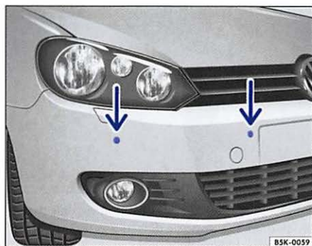
Fig. 133 Park Distance Control system sensors on the front bumper.
