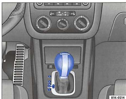
Fig. 84 Section of center console: selector lever
