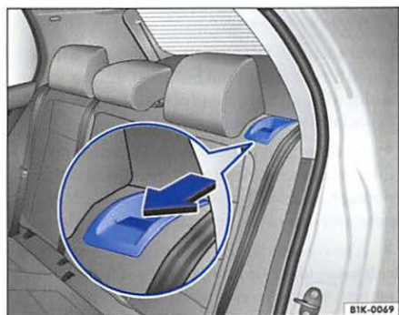
Fig. 55 Rear seat backrest: unlocking
