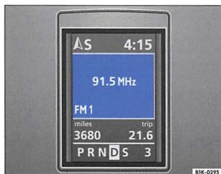
Fig. 13 Display in the instrument cluster: Sound system menu
