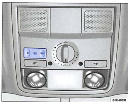
Fig. 39 Section of roof: front interior light
