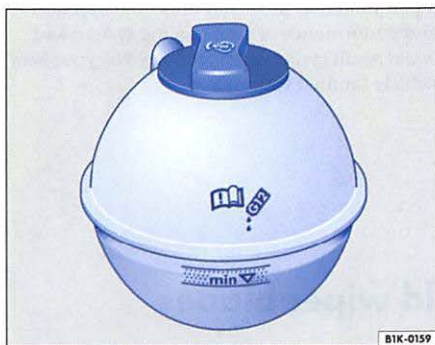
Fig. 8 In the engine compartment: coolant expansion tank
