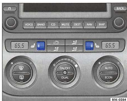
Fig. 53 Detail of instrument panel: thumb wheels for front seat heating
