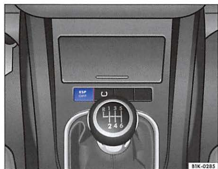
Fig. 1 Detail of center console: Button for ESP
