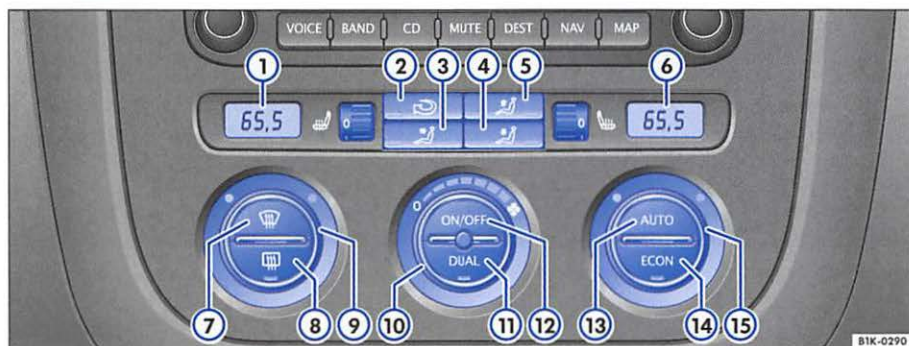
Fig. 76 In the center console: Climatronic controls
