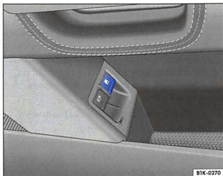
Fig. 2 Detail of the driver door: the fuel filler flap release button
