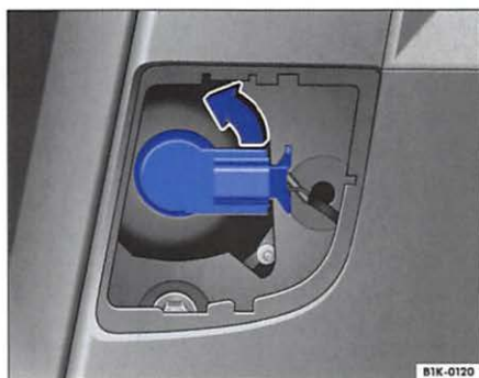
Fig. 43 Remove light bulb holder
