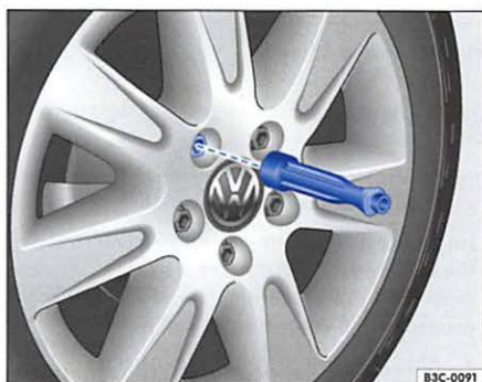
Fig. 28 Changing a wheel: removing the wheel bolts
