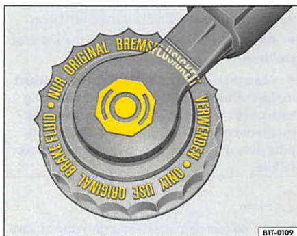
Fig. 14 In the engine compartment: cap for the brake fluid reservoir
