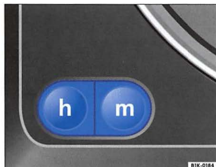
Fig. 4 Section of the instrument cluster: buttons for setting the clock time
