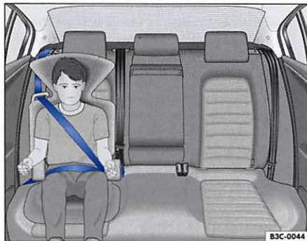
Fig. 33 Child properly restrained in a booster seat on the rear seat
