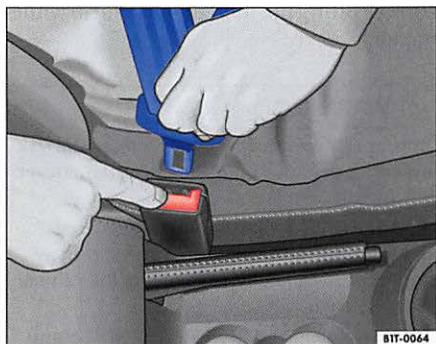
Fig. 19 Releasing the tongue from the buckle
