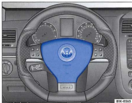
Fig. 21 Location of driver airbag: in steering wheel
