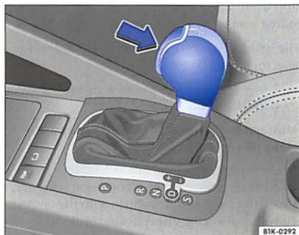
Fig. 83 Section of center console: selector lever with selector lever button
