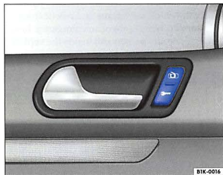
Fig. 27 Detail of the driver's door: central locking button
