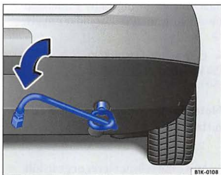
Fig. 48 In the right rear bumper: screwing in the towing eye
