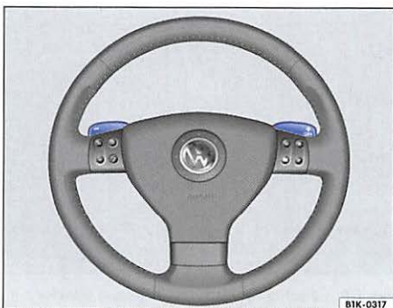
Fig. 86 Multi-function steering wheel: paddles for Tiptronic
