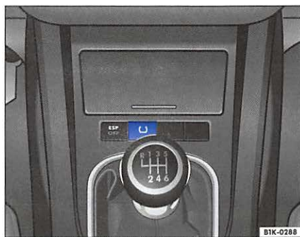
Fig. 16 Section of the center console: button for tire pressure monitoring display
