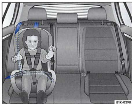
Fig. 32 Smaller child in a properly installed forward-facing LATCH child restraint
