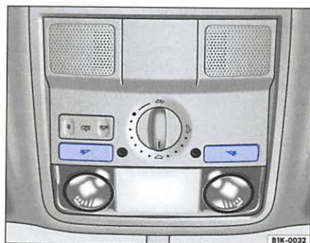
Fig. 40 Section of roof: front reading lights
