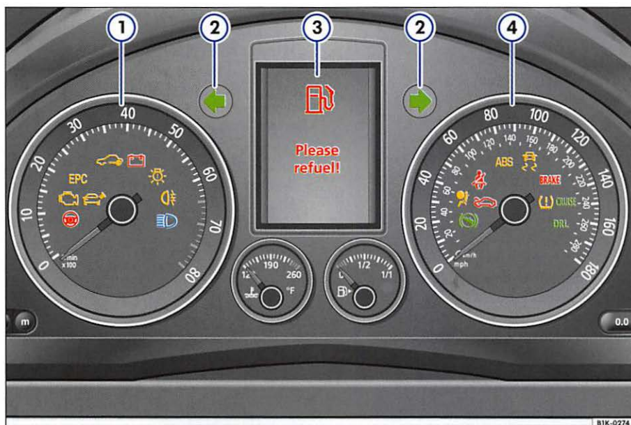
Fig. 2 Instrument cluster with warning lights. Some of the warning lights shown here may be available only on certain models or may be optional equipment. Ask your authorized Volkswagen dealer or qualified workshop for assistance if you have questions.
