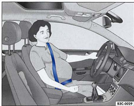
Fig. 15 Safety belt position during pregnancy
