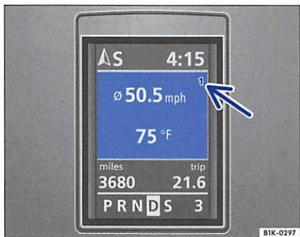
Fig. 17 Display in the instrument cluster: Multi-Function Indicator (MFI)
