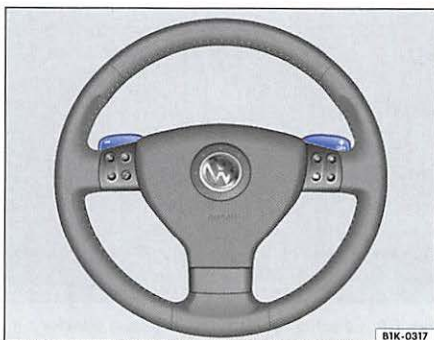
Fig. 86 Multi-function steering wheel: paddles for Tiptronic
