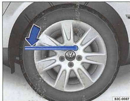
Fig. 24 Changing the wheel: loosening the wheel bolts
