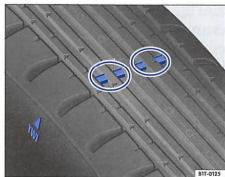
Fig. 17 Tire tread: tread wear indicators (TWI)
