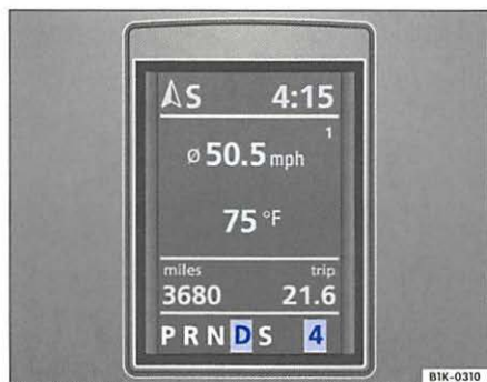
Fig. 87 Selection of instrument cluster: selector lever display with the selector lever in position D and 4th gear
