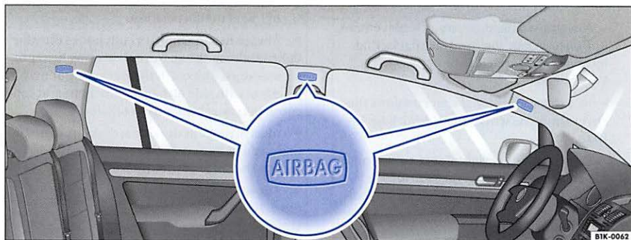
Fig. 28 The Side Curtain Protection™ airbags located above the windows on the sides.
