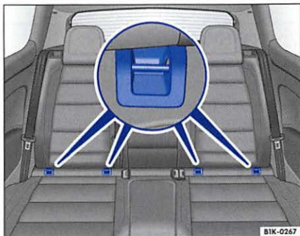
Fig. 36 Illustration of principle: Location of lower anchorages
