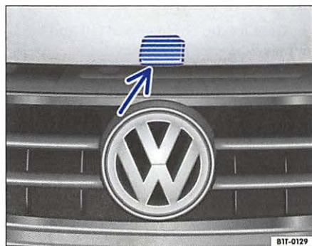
Fig. 5 Detail of the radiator grill: release lever for opening the engine hood
