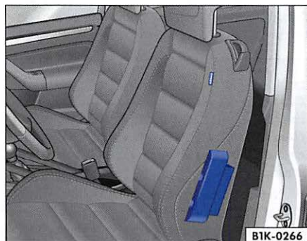
Fig. 26 Side airbag in driver seat
