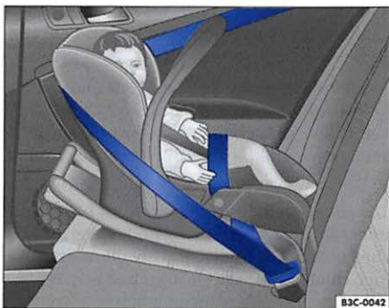
Fig. 31 Rearward-facing infant seat properly installed on the rear seat
