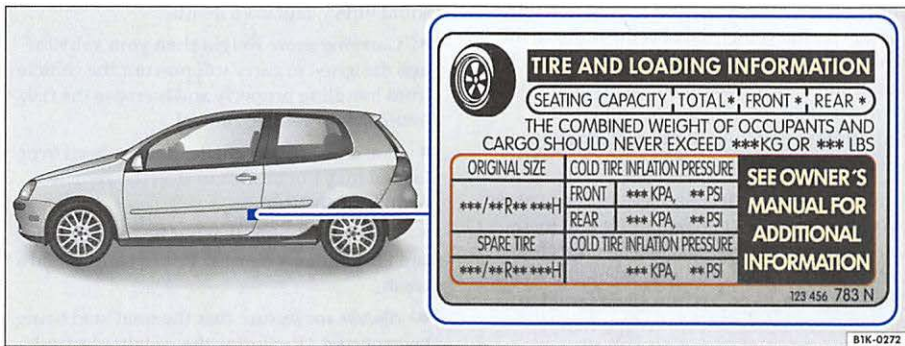
Fig. 15 Approximate location of the tire pressure label on the open edge of the driver's door and example of a tire pressure label
