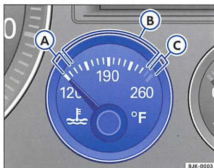
Fig. 4 Section of the instrument cluster: engine coolant temperature gauge
