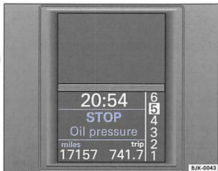
Fig. 9 Warning text in the display of a Midline instrument cluster: STOP Oil pressure
