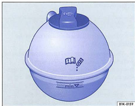
Fig. 7 In the engine compartment: coolant expansion tank
