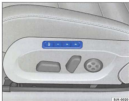
Fig. 46 Memory buttons on the front seat: to save the settings, first press the SET button and then one of the memory buttons, 1, 2 or 3.
