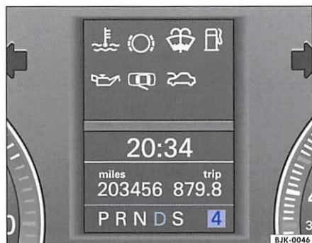
Fig. 82 Section of the instrument cluster: selector lever display with the selector lever in position D and 4th gear
