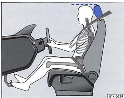
Fig. 2 Correct head restraint position for driver
