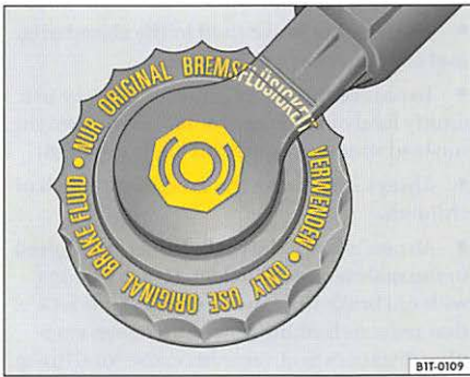
Fig. 12 In the engine compartment: cap of the brake fluid reservoir
