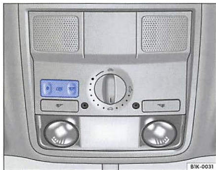
Fig. 28 Section of roof: front interior light
