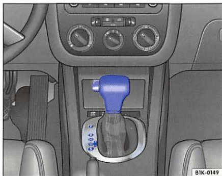
Fig. 80 Section of center console: selector lever with lock button
