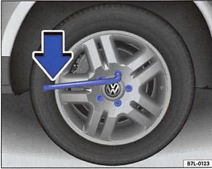
Fig. 23 Changing the wheel: loosening the wheel bolts
