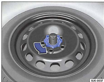
Fig. 21 Under the floor panel: spare wheel secured with a plastic nut.
