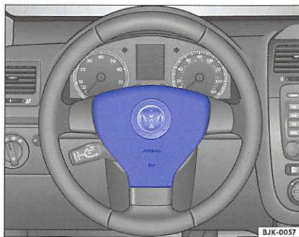
Fig. 21 Location of driver airbag: in steering wheel
