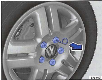
Fig. 20 Detail of wheel: removing the wheel bolt caps
