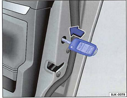
Fig. 29 Using the emergency key to lock the vehicle
