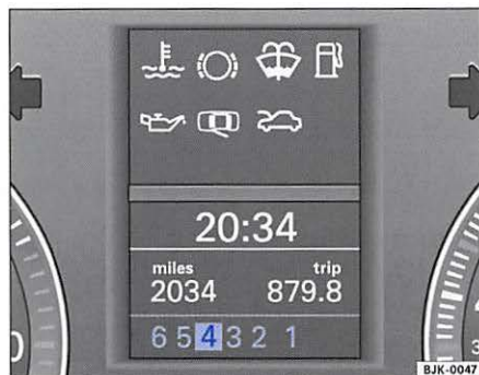
Fig. 83 Section of the instrument cluster: selector lever display in 4th gear selected in the Tiptronic® mode
