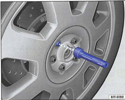
Fig. 27 Changing a wheel: removing the wheel bolts
