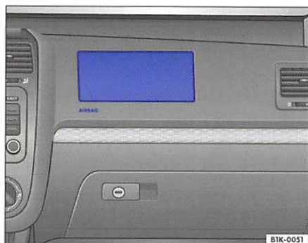
Fig. 22 Location of front passenger's airbag: in the instrument panel
