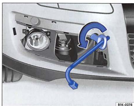
Fig. 46 The front right section of the vehicle: screwing in the towing eye
