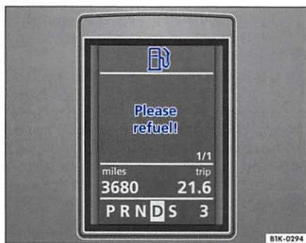
Fig. 8 Warning symbol and warning text in the display of the instrument cluster
