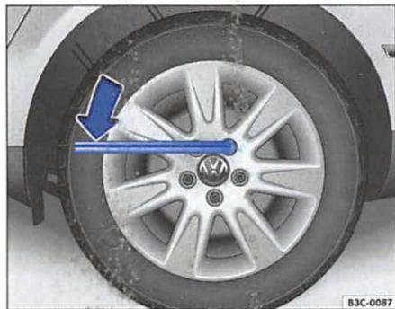
Fig. 24 Changing the wheel: loosening the wheel bolts
