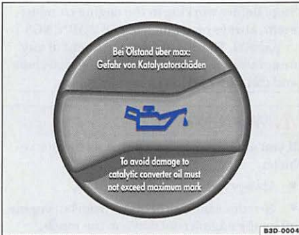
Fig. 7 In the engine compartment: engine oil filler cap
