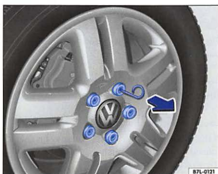
Fig. 23 Detail of wheel: removing the wheel bolt caps
