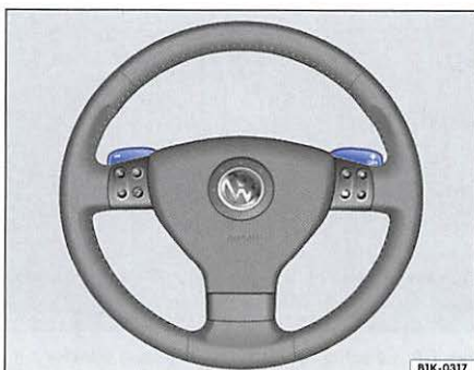
Fig. 86 Multi-function steering wheel: paddles for Tiptronic
