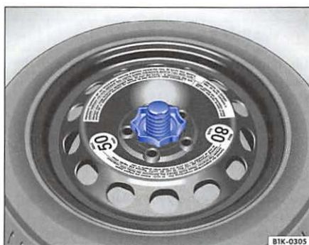
Fig. 22 In the luggage compartment: handwheel for securing the spare wheel
