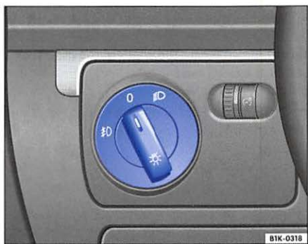
Fig. 35 Section of instrument panel: switch for the headlights, automatic headlight control and front fog lights
