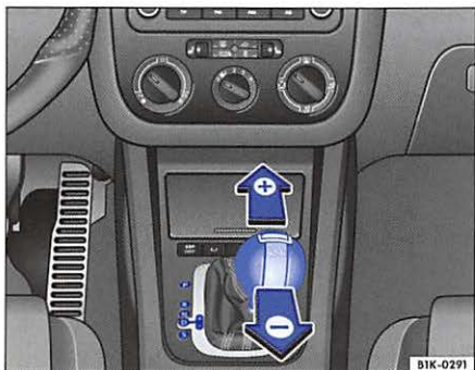
Fig. 85 Section of the center console: automatic transmission in Tiptronic position
