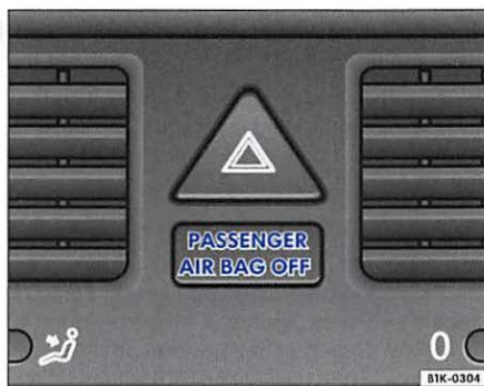
Fig. 25 Section from the instrument panel: PASSENGER AIR BAG OFF
