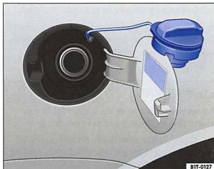
Fig. 3 Open fuel filler flap with filler cap attached to the flap
