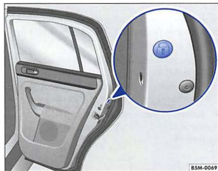
Fig. 29 There is an emergency lock (covered by a weatherstrip) in the edge of the left rear door
