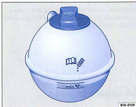
Fig. 8 In the engine compartment: coolant expansion tank
