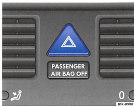
Fig. 37 Section of instrument panel: switch for the emergency flasher
