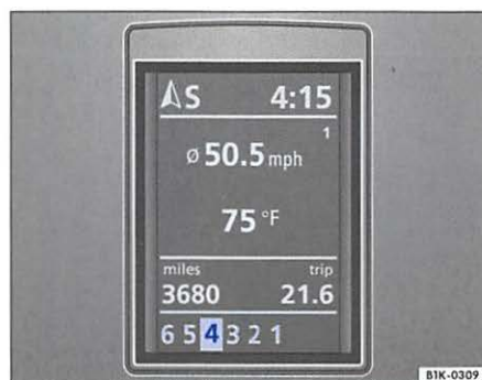
Fig. 88 Selection of instrument cluster: selector lever display in the 4th gear selected in the Tiptronic mode
