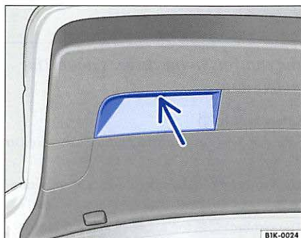
Fig. 32 Section of the rear lid interior trim: recesses for closing
