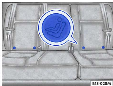
Fig. 1 The illustration above shows the location of the circular seat markings for the lower anchorages for the outboard rear seating positions.
