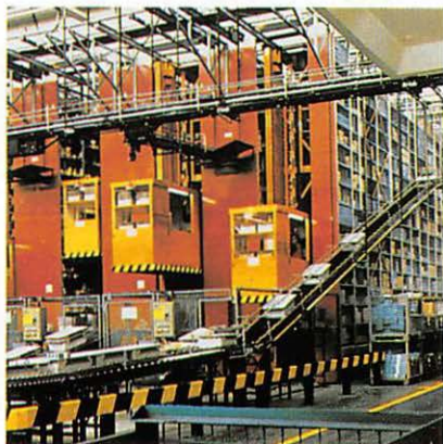
The central parts facility in Kassel, West Germany has automatic parts retrieval systems to expedite parts orders worldwide.
