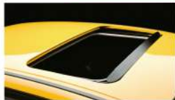
▲ An optional power tilt and slide sunroof with a built-in air deflector helps reduce wind noise, and makes every drive a little more refreshing.
