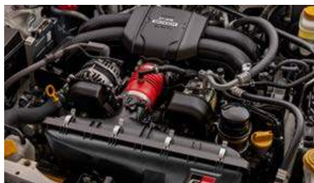
GR air intake system
