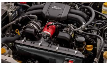
GR air intake system
