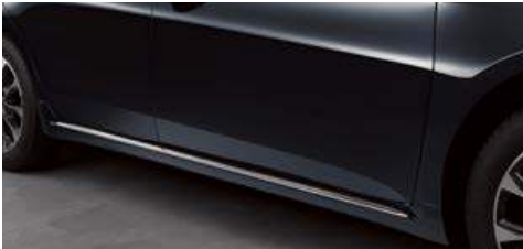
Lower door molding
